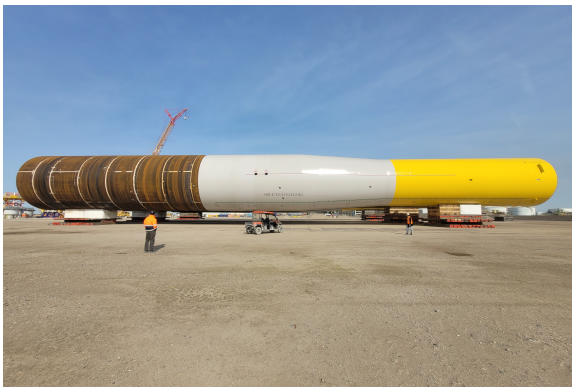
Figure 2.12: Monopile made of S355 steel, partly covered with a coating (right).
