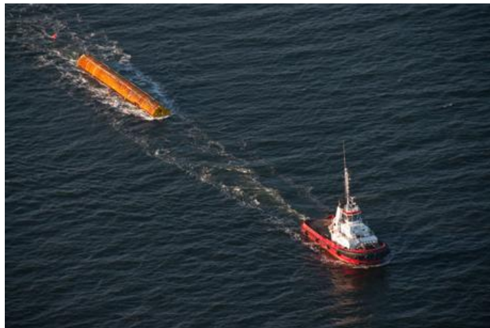
Figure 2.7: Floating monopile towed by a tugboat [20].
