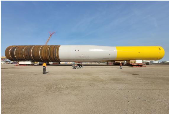
Figure 1.2: An image of a monopile made at SIF.
