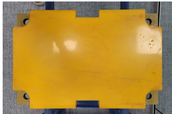
Figure 2.13: A polymer friction pad currently used by TWD for seafastening monopiles.
