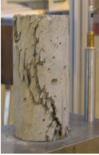
(a) Failure mode of UHPCFRC
