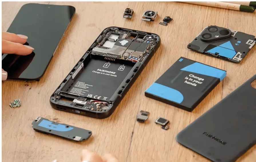
fig. 107 Color-coded components for intuitive installation (Fairphone, 2023)
