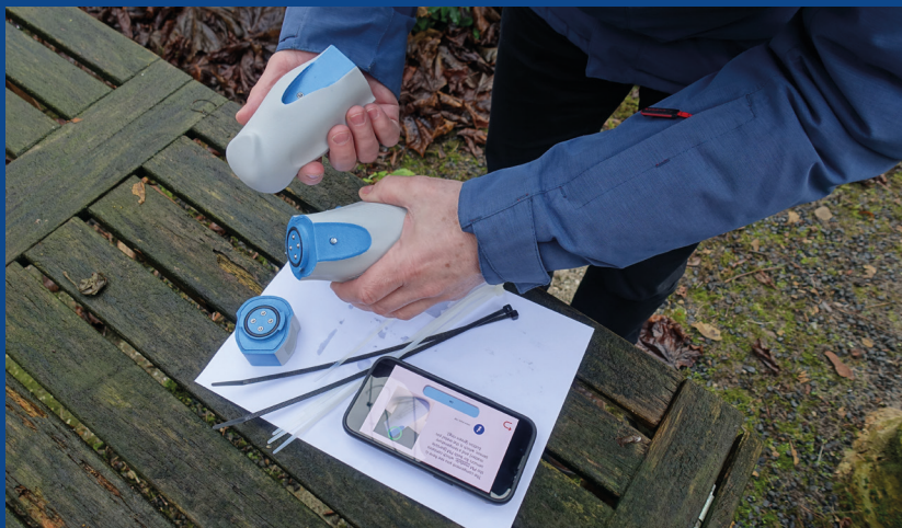
fig. 176 Interactive manual that makes use of the phone's sensors to assist in optimal placement
