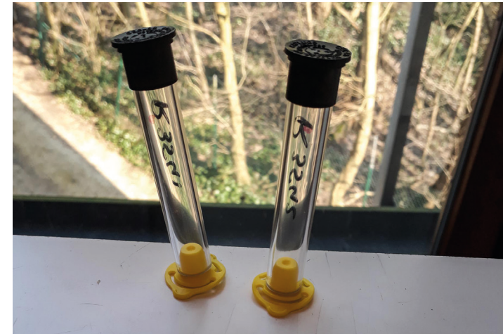
fig. 152 An example of a user error in the first “CurieuzeNeuzen” project: participants forgot to close off their Palmes tubes to end measuring, before returning them (CurieuzeNeuzen, n.d.-b)
