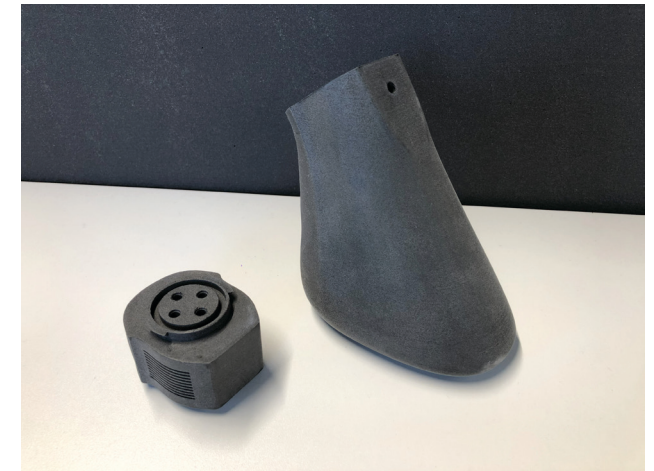
fig. 162 First 3D print, produced using SLS
