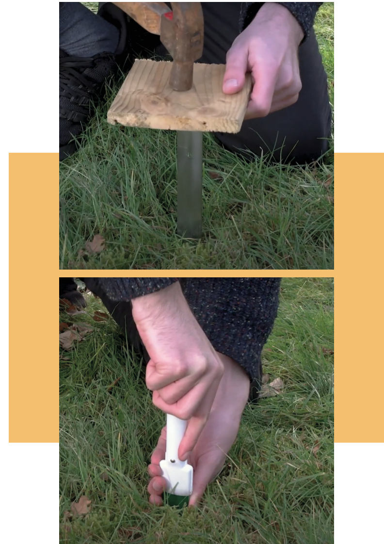
fig. 12 Additional tools (hammer, blade and wood) required to install the instrument in the "CurieuzeNeuzen in de Tuin" project (CurieuzeNeuzen, 2022)
