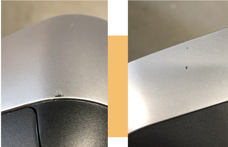
fig. 115 Damaged paint causing the base material to be revealed
