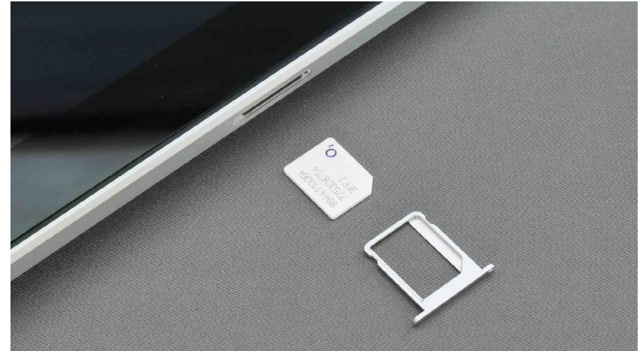
fig. 138 Example of ポカヨケ, an asymmetrically shaped SIM card that can only be inserted in a single way
