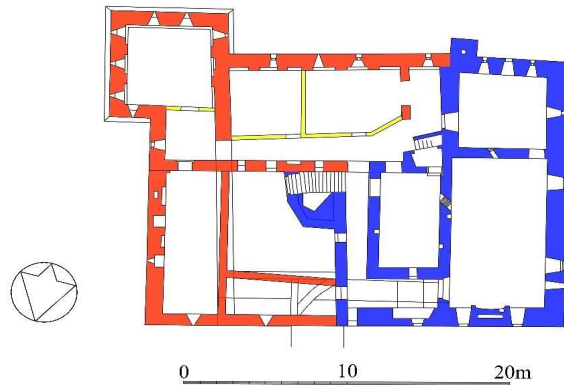
Figure 38- Representation of the two phases of the castle, the blue from 1571 and the red from 1616 (Viersen, 2014)
