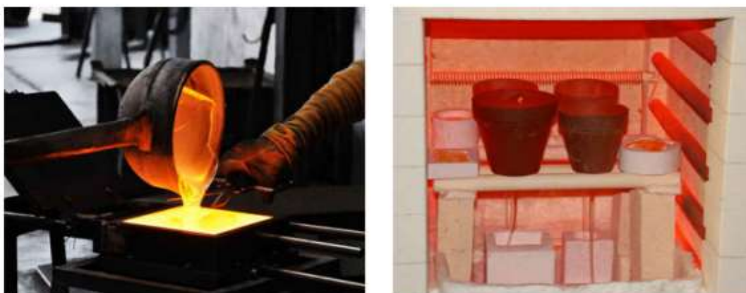
Figure 5- Hot pour (left), kiln-cast (right) (Oikonomopoulou, 2019)
