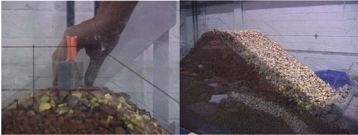
Figure 3.3 Installation of filter layer
