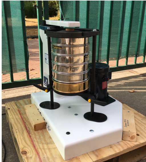
Figure 2.4: Set-up ball-pan hardness test
