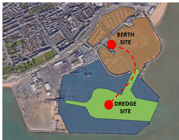
Figure 5.9: Ramsgate area with dredge and berth sites and the route shown with dashed red line
