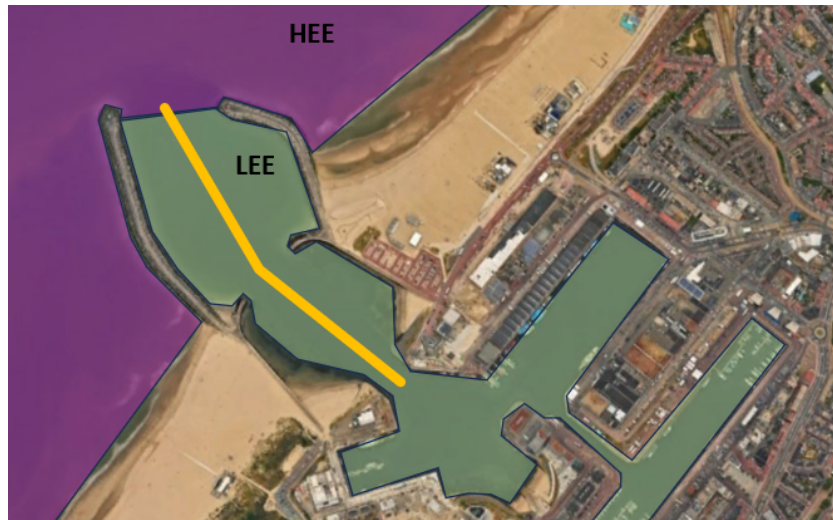
Figure 2.2: Example of Low Energy Environment (green), High Energy Environment (purple), and a discharge channel (yellow) (Google Earth, 2024)
