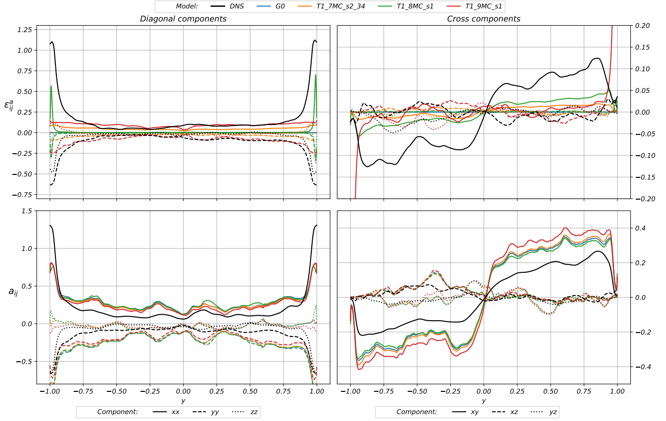
Figure 17. Comparison of a_{ij} and \varepsilon_{ij} profiles of models T2_7MC_s2_34, T1_8MC_s1 and T1_9MC_s1. G0 model is provided as reference.
