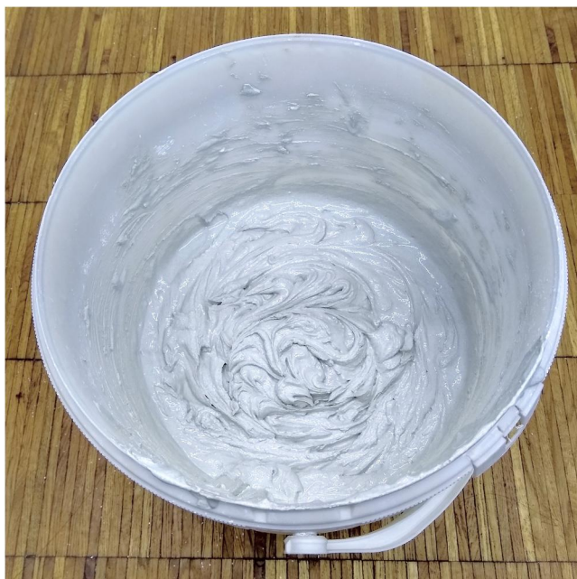
Figure 7. Photograph of the saturated electrolyte stabilized in a clay. The consistency is that of a wet mud or gelato.
