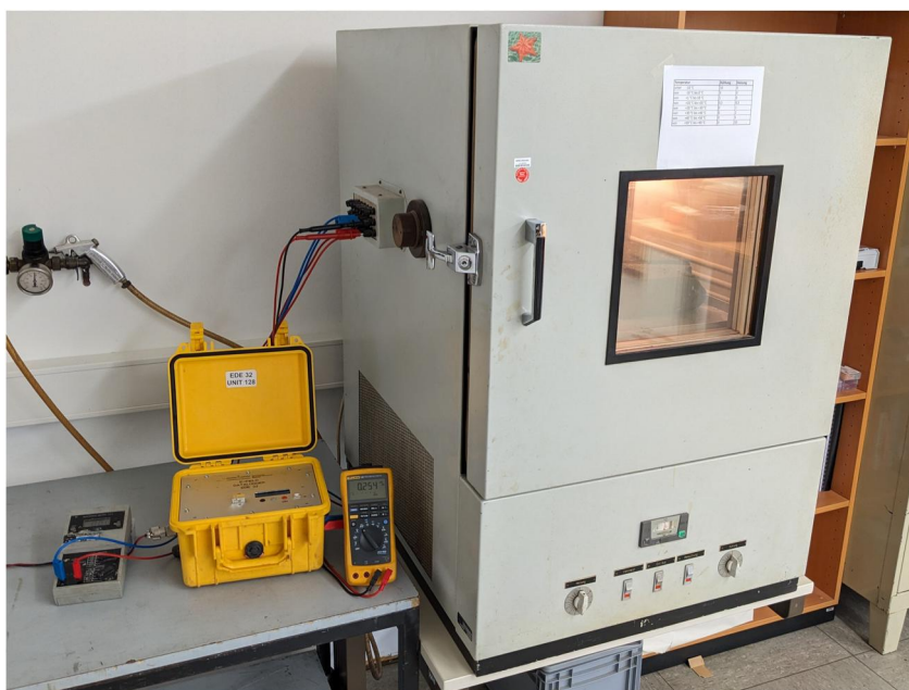
Figure 9. Photograph of the (Vötsch) temperature-controlled climate chamber where measurements of the temperature sensitivity of the electrodes were carried out.
