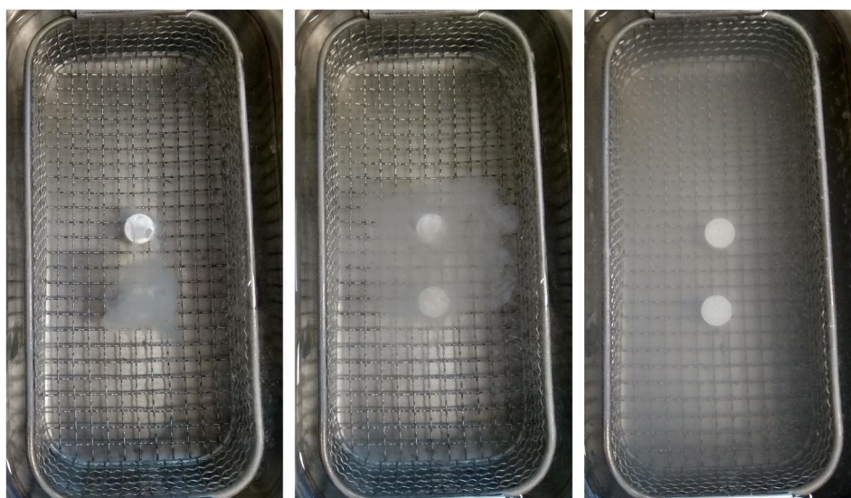
Figure 6. Photograph of the process of cleaning the ceramic pellets in a warm ultrasonic bath. The photographs show the time progression from left to right (0 s, 4 s, 200 s; note that the water has become clouded with contaminants).
