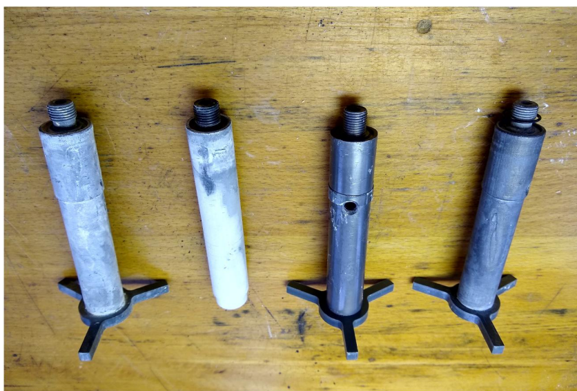
Figure 4. Photograph of the lead tubes before and after cleaning. Due to the modular design, the lead tube can be removed, cleaned, and re-installed with ease. Two used or dirty tubes are on the left and two clean tubes are on the right. The plastic stabilizer at the bottom keeps the tube in position in the pot and helps preserve the shape.
