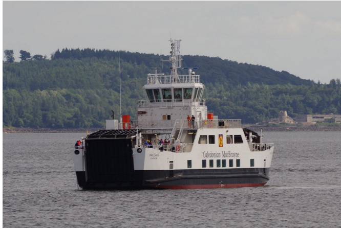
Figure 2.18: Ferry with electrical propulsion and hybrid power supply.
