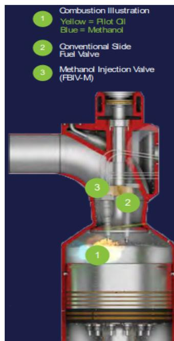
Figure 2.1: Illustration of a combustion chamber, with methanol injection valve [19]
