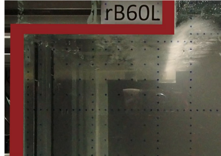
(e) Impact Type V: for BL and DL. Intermediate entrapped air, far from wall
