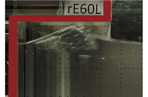
(f) Impact Type VI: for EL and FL. Double peak, singular air pattern
