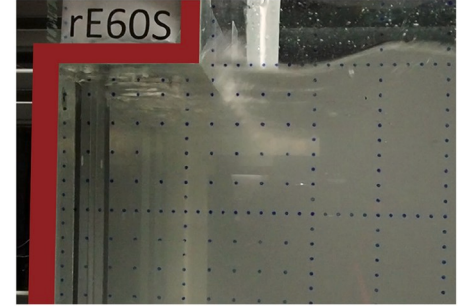
(c) Impact Type III: for ES and FS. Reduced entrapped air, distributed
