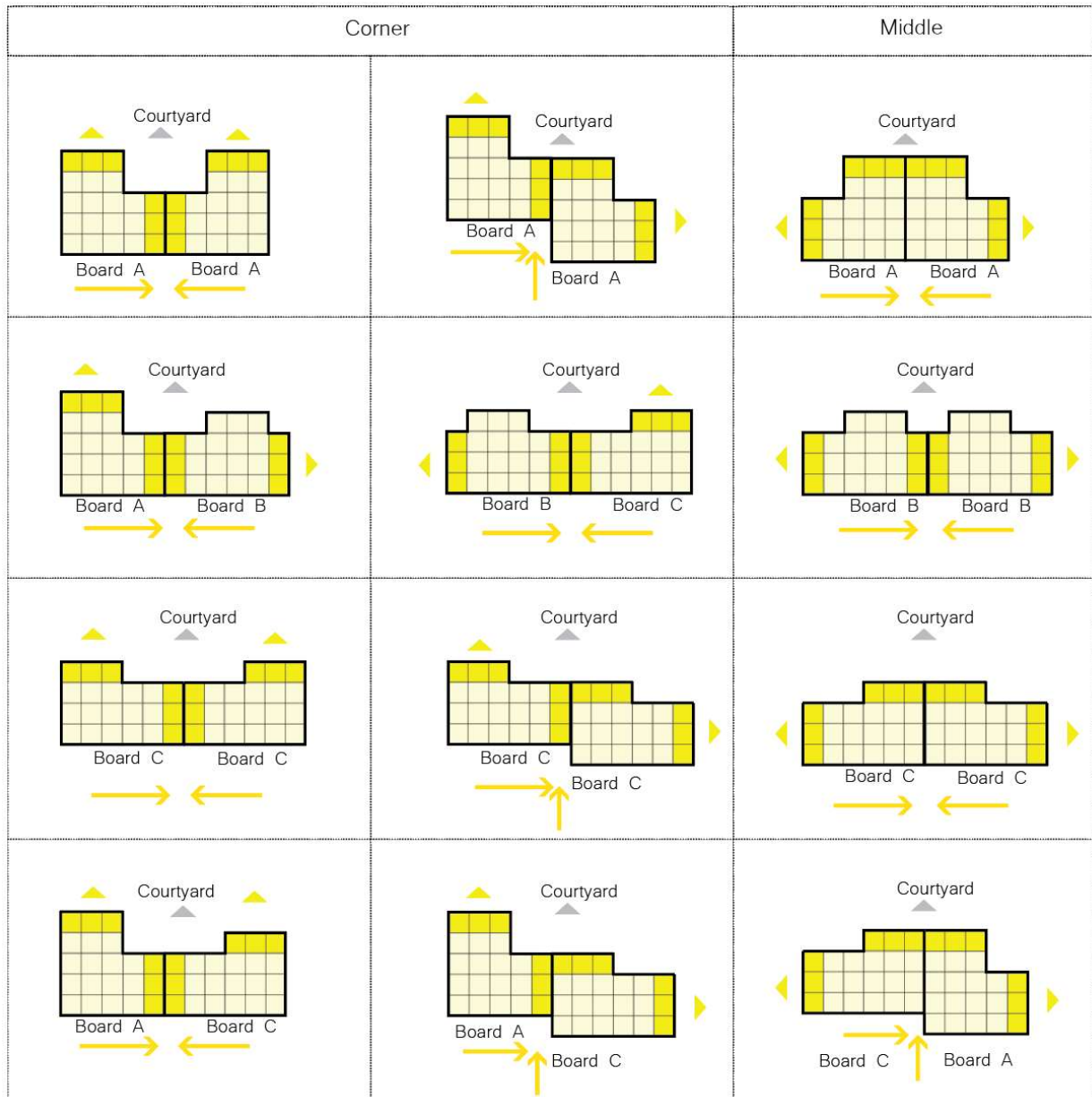
Figure 94: Connection possibilities of various board types. By Author, 2021
