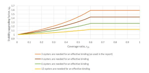
Figure 8.2: Effect of different numbers of binding oysters on the relationship between the coverage ratio and the stability upgrading factor for stone grading 10-60 kg
