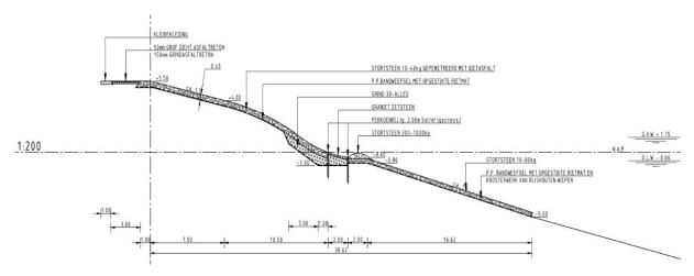
Figure E.7: Schematic overview of the revetment at location 15
