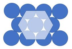
Figure 4.1: Hexagonal circle packing in 2D (based on A. Thue, 1890)
