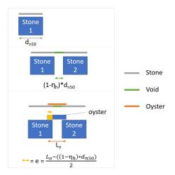
Figure 4.2: Effective settling distance from the edge, side view
