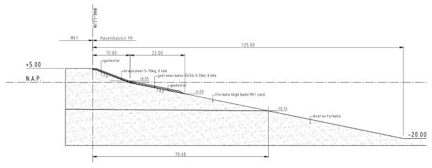
Figure E.3: Schematic overview of the revetment at location 5
