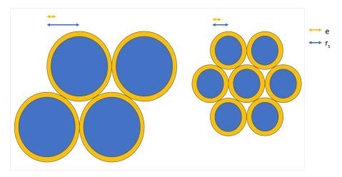
Figure 4.3: Ratio between the total area and the effective settling distance for various stone dimensions, top view
