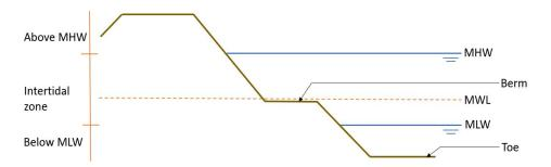
Figure 3.4: Schematic drawing of a revetment in vertical space
