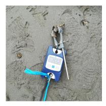
Figure 4.6: Clamp and tensile force gauge used for pulling C. gigas from the surface
