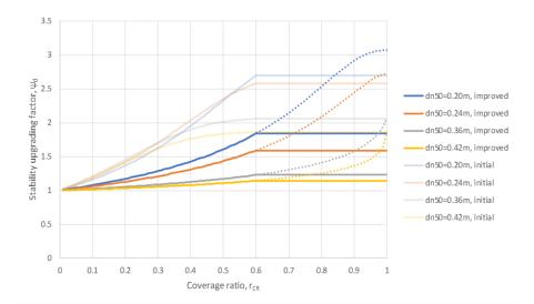
Figure 9.1: Improved relationship between the coverage ratio and the stability upgrading factor for different nominal stone diameters. With dashed lines showing the model without upper limit
