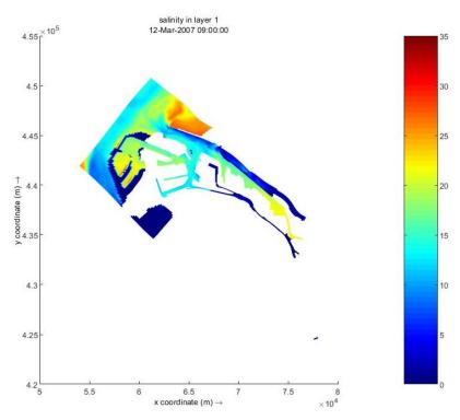
Figure 3.3 (c) Scenario 3: HWS, during a high water discharge at Lobith of 5700  $\mbox{m}^{3}/\mbox{s}$
