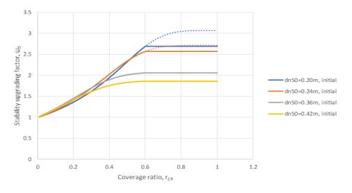
Figure 4.5: Initial relationship between the coverage ratio and the stability upgrading factor for various nominal stone diameters
