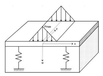
Figure 2.2: Schematization of the load impact on an impermeable revetment (De Looff et al., 2006)
