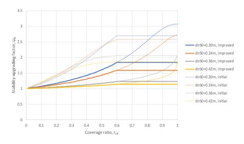
Figure 4.8: Improved relationship between the coverage ratio and the stability upgrading factor for different nominal stone diameters
