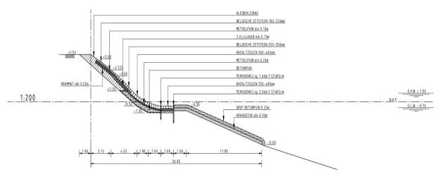
Figure E.5: Schematic overview of the revetment at location 12
