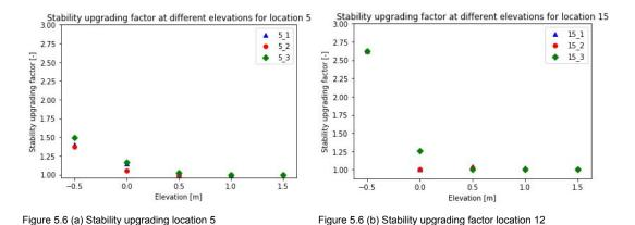
Figure 5.6: Calculated stability upgrading factor from the observed absolute and effective number of exposed stones
