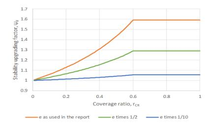
Figure 8.3: Effect of different effective settling distances of oysters on the relationship between the coverage ratio and the stability upgrading factor for stone grading 10-60 kg
