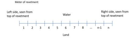
Figure 5.1: Overview of allocation of numbers to areas at a revetment
