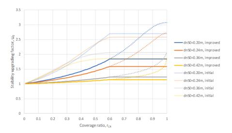
Figure 9.2: Validation of the connectivity model with measurement outcomes for different coverage ratios and a nominal stone diameter of 0.20 m and 0.30 m
