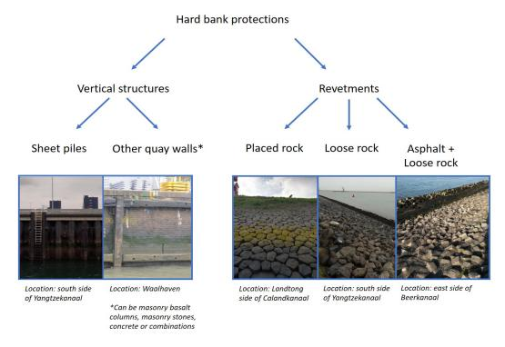
Figure 1.2: Schematic representation of the types of hard bank protections used in the port area, based on Paalvast (2017)
