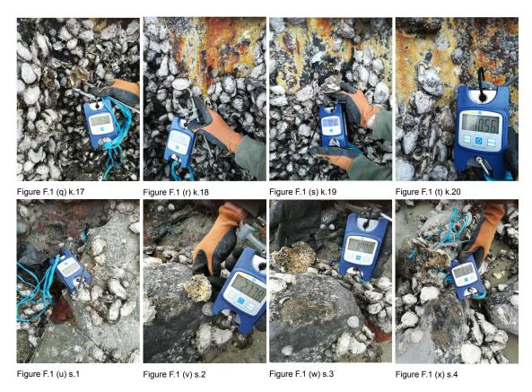
Figure F.1: Pictures taken during measurements of oyster attachment
