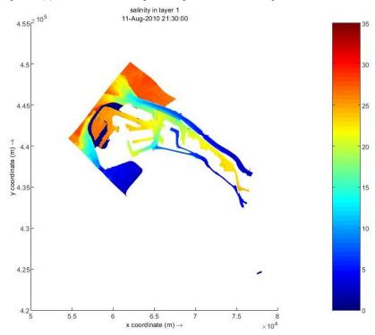
Figure 3.3 (b) Scenario 2: LWS, during an average normal water discharge at Lobith of 2300  $\mbox{m}^{3}/\mbox{s}$
