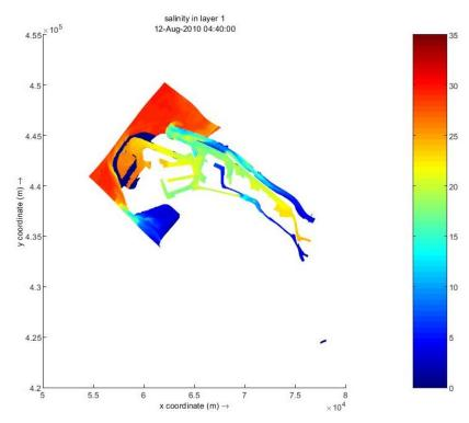
Figure 3.3 (a) Scenario 1: HWS, during an average normal water discharge at Lobith of 2300 m³/s
