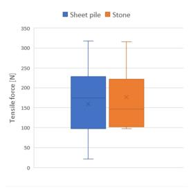
Figure 4.7: Tensile force of C. gigas attachment to sheet piles and stones
