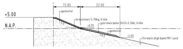
Figure 2.1: Schematic overview of the revetment at location 5 (see Figure 3.8 for the exact position of location 5)
