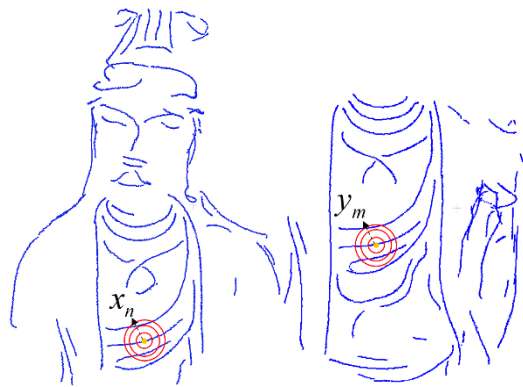
Figure 9. Schematic diagram of curve constraints: red circles indicate neighborhood areas of three scales from two point clouds.
