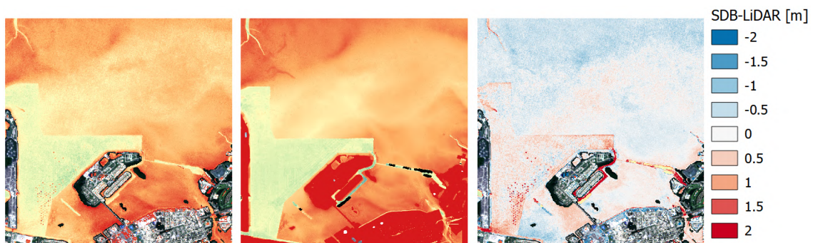
Figure 4.20: Left: SDB, middle: LiDAR, Right: Difference between SDB and LiDAR [m], (Key West, FL)
