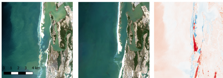
Figure 3.8: Four years of morphological development (2016-2020) captured with Sentinel-2 satellite images of St. Louis, Senegal. Left: 2016, middle: 2020 and right: the difference of green signal between two images. Red areas show locations of sedimentation, blue areas is where erosion occurred
