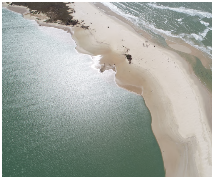
Figure 2.2: Sun glint on a drone image appears as a bright spot in the water
