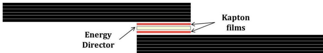
Figure 2.11: Isolation of the energy director using Kapton films [16]
