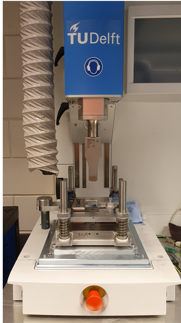
Figure 3.9: Hermann Ultrasonic Welder fitted with lap-shear joint fixture
