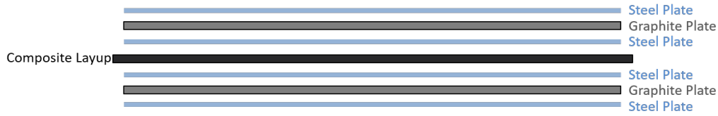
Figure 3.4: Side view of layup in stack for pressing
