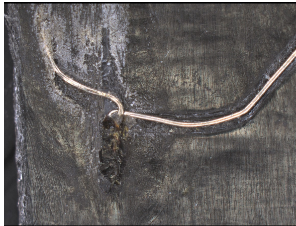
Figure 5.1: Microscope photograph of a thermocouple tip after welding CF/PEEK 1ply H
