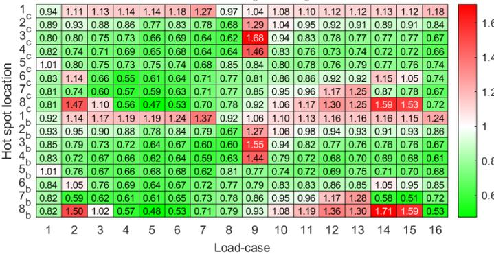
Ratio with/without LMF of accumulated fatigue damage
