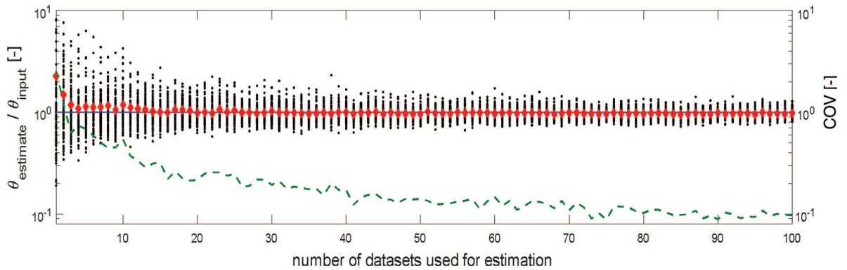
Figure 1. Example analysis investigating the accuracy in calculating  $\theta$  as a function of the number of datasets. Each dot is a single estimation of  $\theta$ , normalized by the input  $\theta = \theta_{input}$ ; the horizontal line equal to 1 is the normalized input  $\theta$ ; the red diamonds are the calculated average from the individual estimates; and the broken line is the calculated coefficient of variation ( $COV = \sigma/\mu$ ) of the estimated  $\theta$ .
