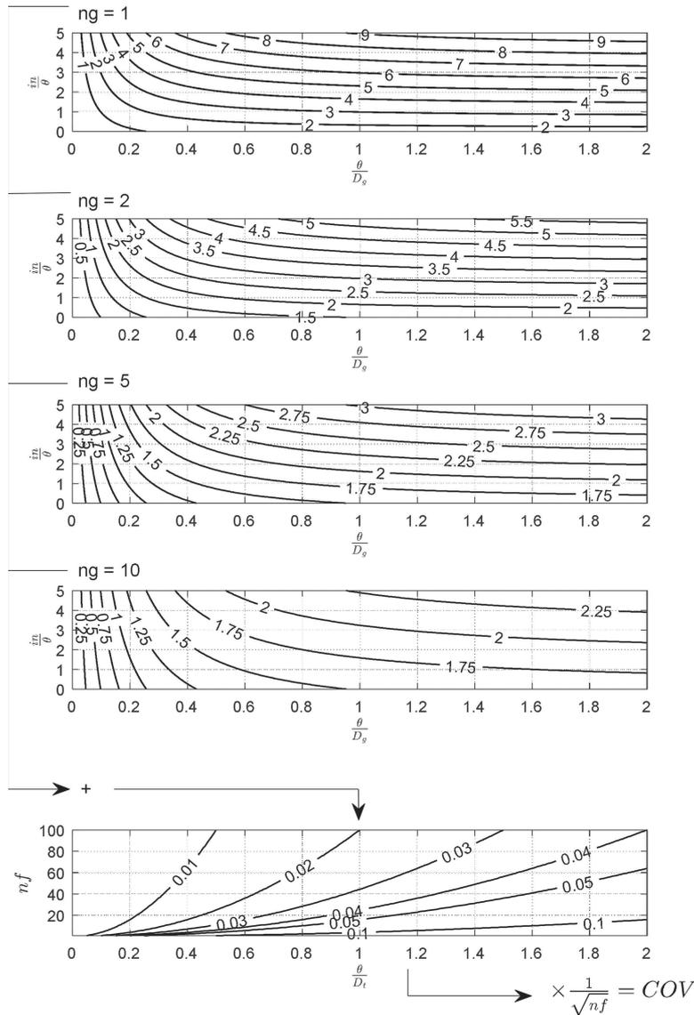
Figure 2. Method of estimating COV of the scale of fluctuation using groups of data.
