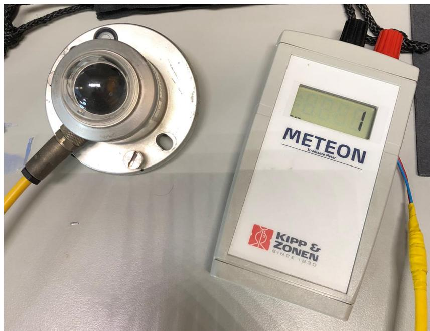
Figure 34: Solar irradiance meter used in the solar box of [Figure 33](#).
