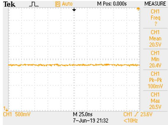
Figure 16: The input voltage of the converter with the capacitor
