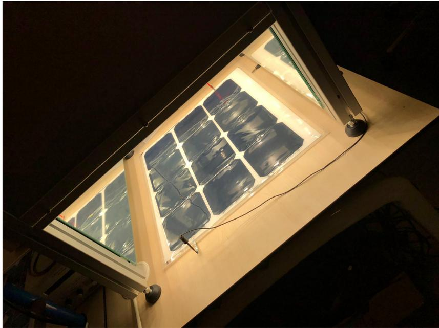
Figure 33: Solar box and PV-module for the practical measurements.
