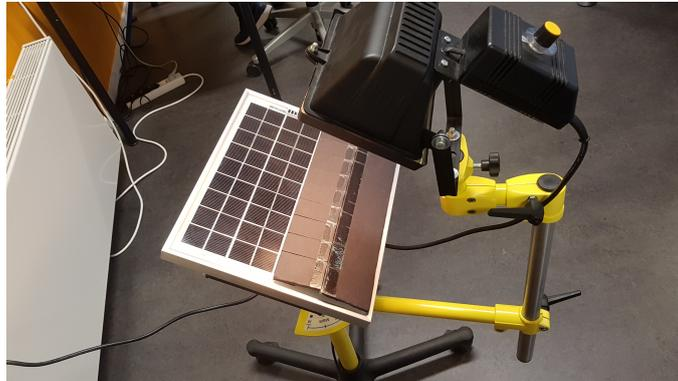
Figure 36: ST014 under partially shading
