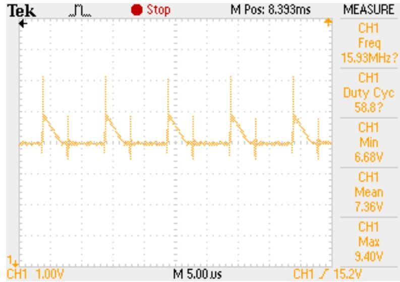
Figure 30: Output voltage of first SEPIC (Figure 16). Input: 4V, 59% duty cycle.
