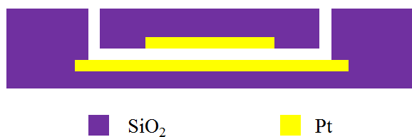
Figure 1.7: Schematic illustration of nanogap device assembly proposed by Lemay et al. [58].
