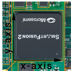
Figure 5.12: SmartFusion2 Starter kit reference for the XY-table measurements.
