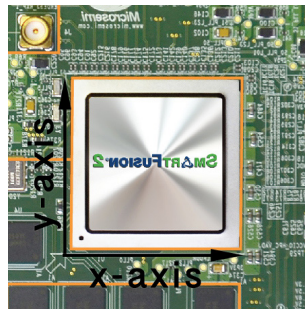
Figure 5.19: SmarFusion2 Advanced kit reference for the XY-table measurements. Measurement on the back, which makes the images flipped horizontal from the front.
