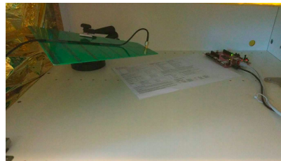
(b) The attack set-up inside the shielded box.
