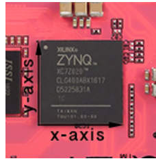
Figure 5.1: PYNQ-Z1 reference for the XY-table measurements.
