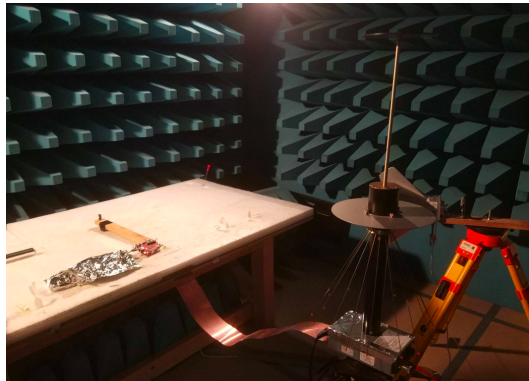
Figure 3.14: The set-up in the anechoic chamber using a discone antenna and batteries.
