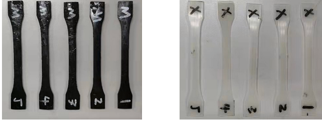
Fig. 11. Dumbbell shape of MDPE (left) &amp; XLPE (right).
