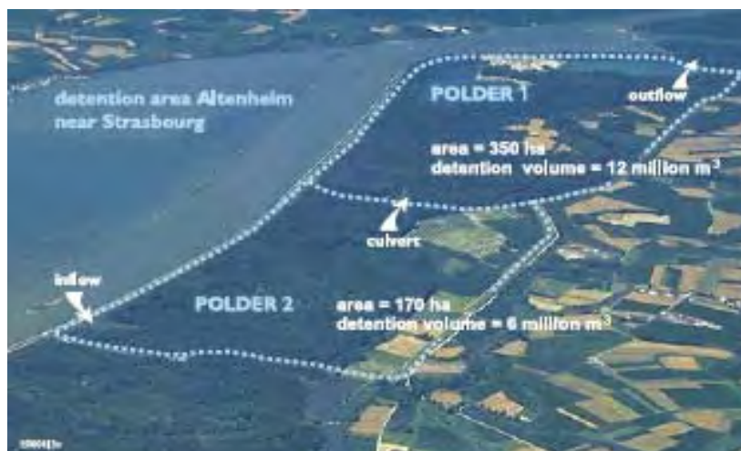
Figure 4.3 Layout of a detention area along the Oberrhein (Source: Hochrhein)
