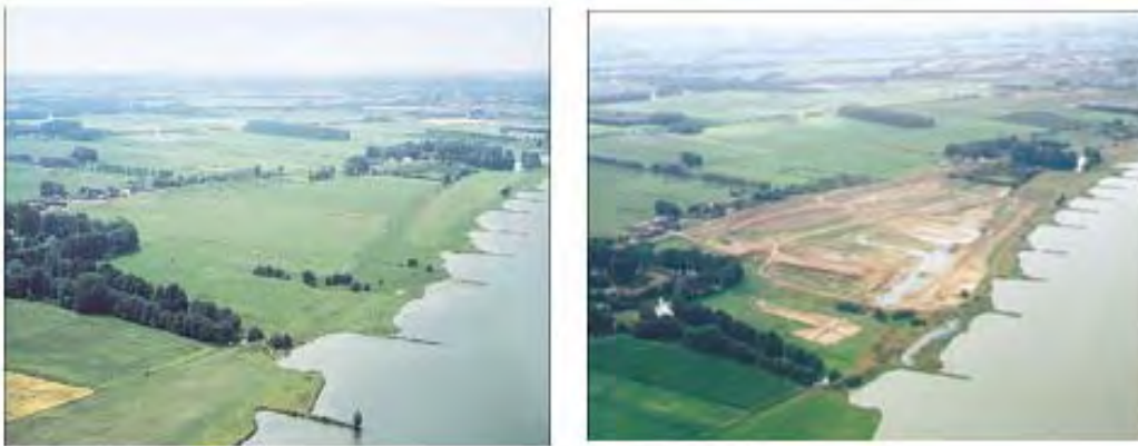
Figure 4.7 excavation and nature development in the Baarsemwaard flood plain along the Neder-Rhine Left: before implementation Right: in progress (1999) (Source: Draex)
