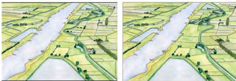
Figure 4.9 Setting back the dikes locally (Source: K.Nuijten)
