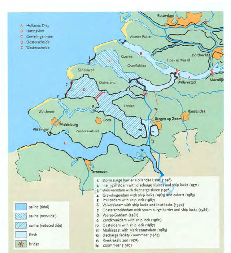
Figure 3.14 The revised plan of 1986 for the Delta project with the names of the completed and newly designed work
