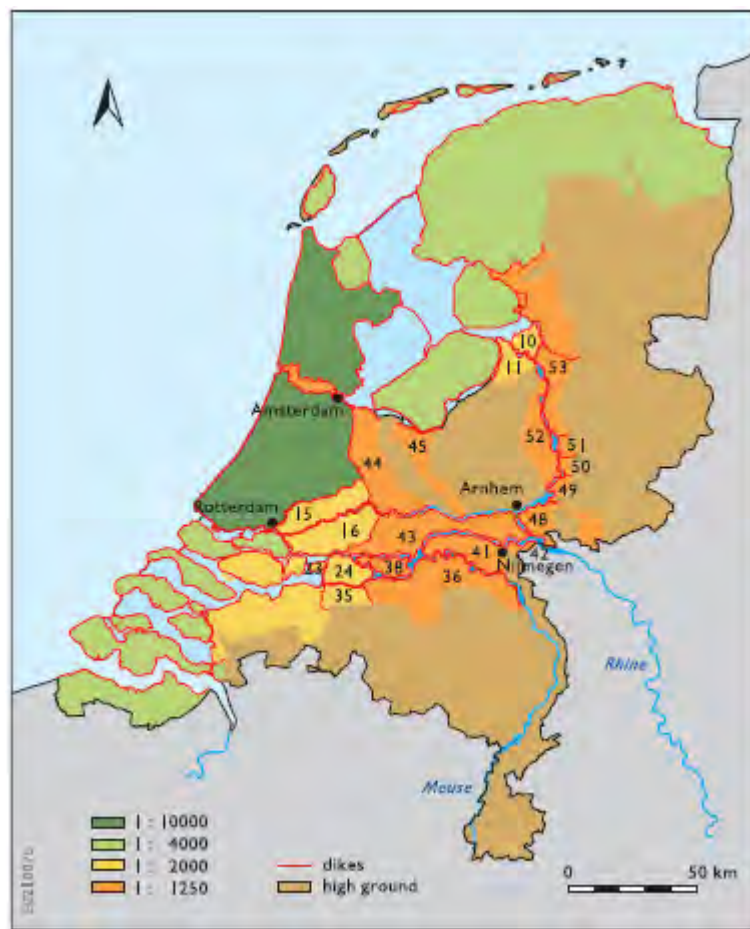
Figure 3.7 dike rings and safety levels along the lower Rhine River
