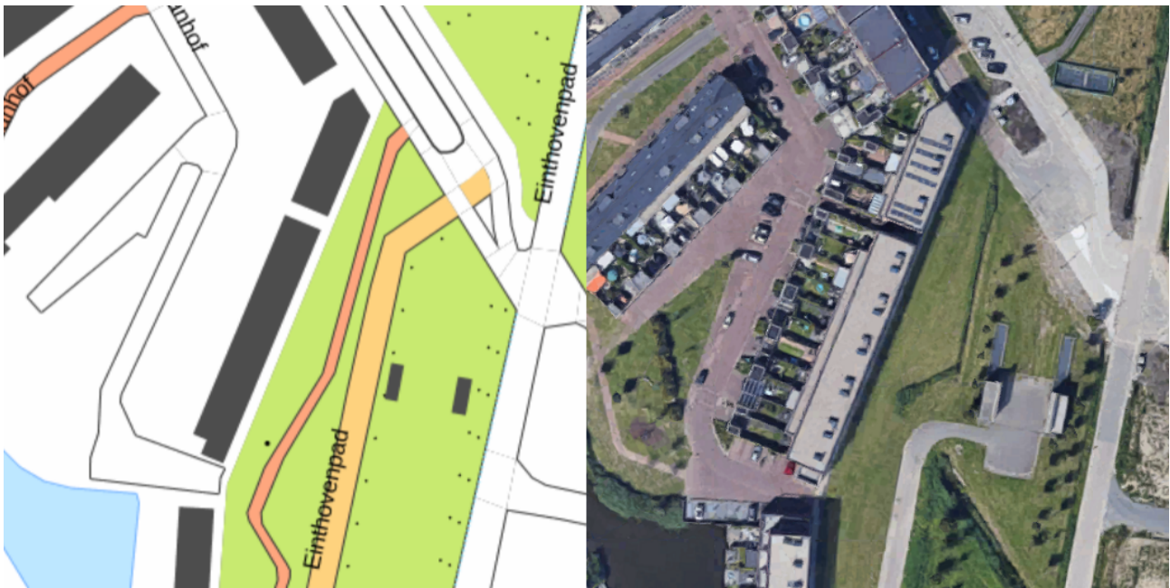
Figure 6.2: Comparison of the used topographic data (left) with satellite images (right) provided by Google, Aerodata International Surveys, and Maxar Technologies (2021). On the left image, white areas represent other land usage, black areas indicate the presence of buildings and green areas indicate grassland.
