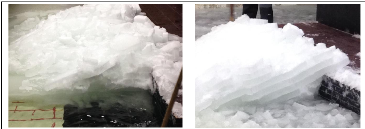
426 Figure 3-4. Cross section photos taken at the end of the ice encroachment model tests with 'soft' and 427 'strong' ice (right and left image respectively). Layering of ice is clearly evident in the strong ice, 428 whereas soft ice pile is composed of broken and randomly orientated ice.
