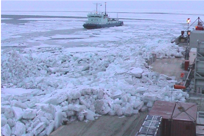
49 50 Figure 1-1. Example of Ice Encroachment ride-up event in Caspian Sea. Source: Mckenna et al. (2011).
