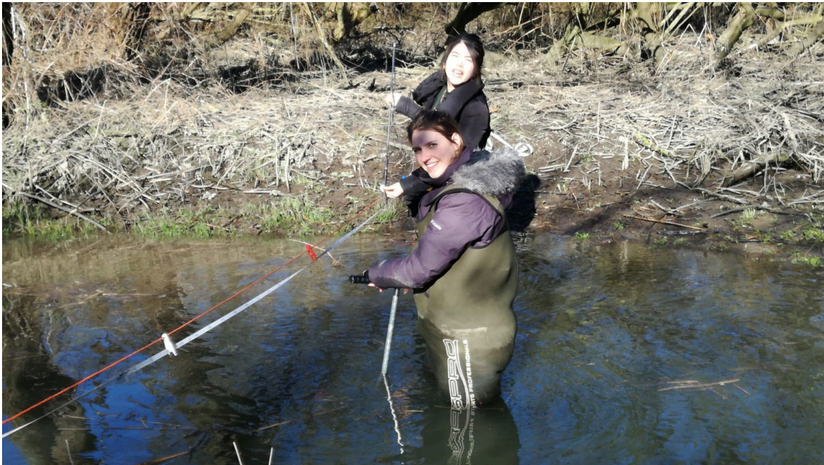
Figure 4.6: Propeller measurement during high water
