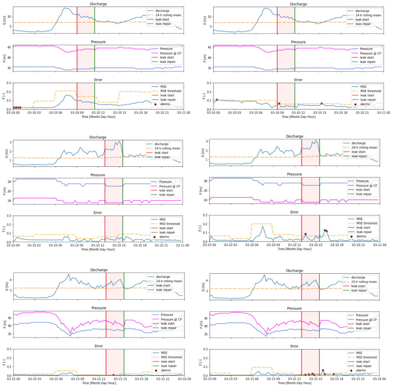
Figure 11: Fire hydrant leak tests in DMAs Beta (top), Delta (middle) and Zeta (bottom).. Left sub-figures show the result of running the model with two pressure signals as input in scenario A. Right sub-figures show the result of running the model with all the pressure sensors available as input after utilizing transfer learning in scenario C. Sub-figures in top row show the discharge at the inflow of the DMA. The middle row sub-figures show the pressure signals at the inflow of the DMA and the critical point. The lower sub-figures show the MSE (error) function, the variable error threshold, the start and repair time of the fire hydrant leak tests and the raised alarms.
