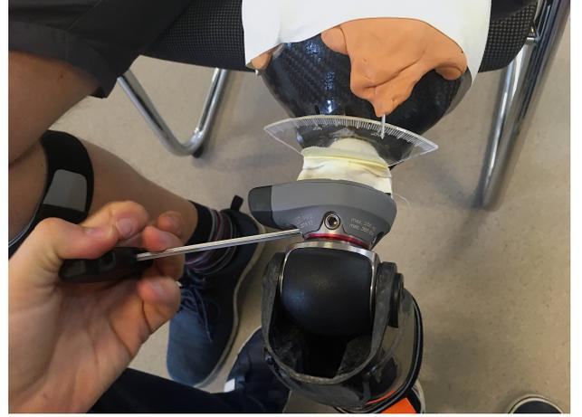
**Fig. 14:** CPO adjusting the VR/VL-A by turning the screw on the right side of the adapter. Further, to be seen, the plate and indicator above the knee joint to trace the changes in the I/O-RA alignment.
