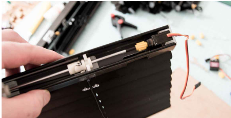
FIG. APP.D.8 Integration of a servo motor in the venetian blinds of the sun protection
