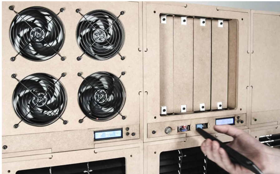
FIG. 5.13 The ventilation flaps close due to noise pollution and mechanical ventilation is activated
