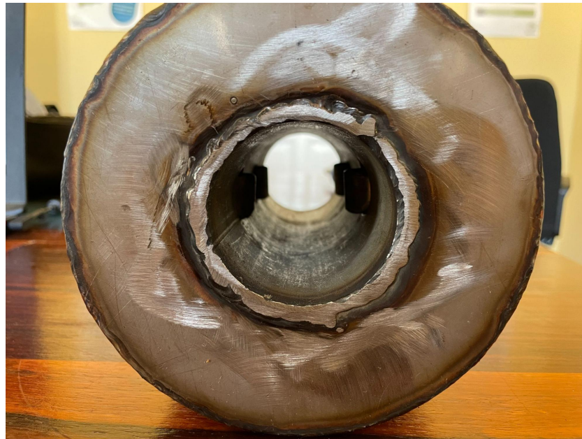
Figure A.4: The inside of the female part where the latches can be seen
