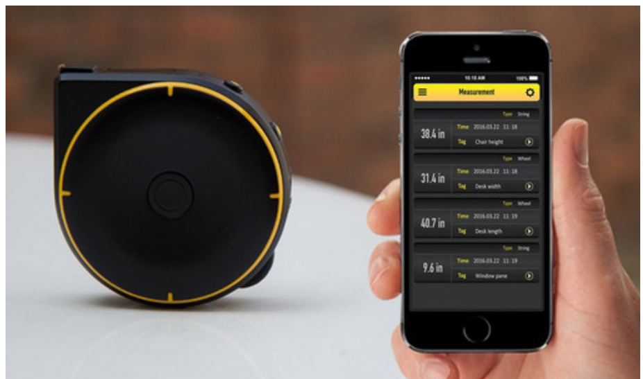
Figure 21. Digital tape measure Bagel connect to its application [10]
