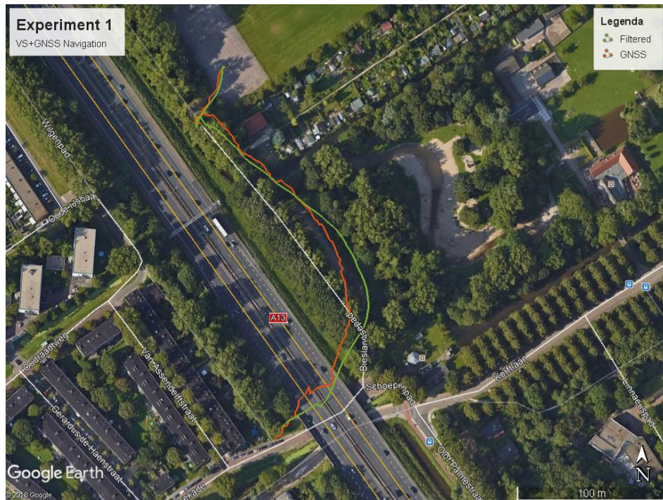
Figure 6-3: This figure shows the GNSS data as well as the filtered output. The vehicle drove along the Bieslandsepad (the path hidden behind the treeline).
