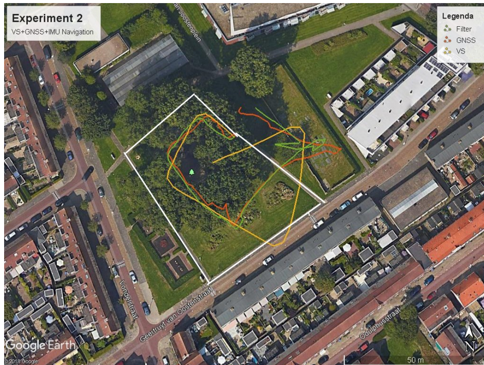
Figure 6-6: This figure shows the results of the filter in green, the GNSS data in red and the VS only result in yellow. The actual travelled path is displayed in white
