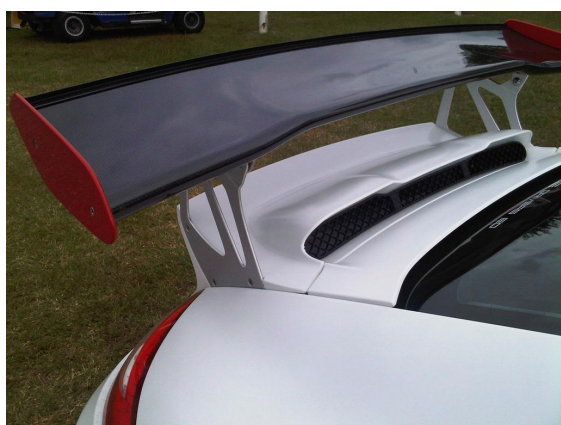
Figure 1.5: Gurney flap on Rennspeed modified Porsche
