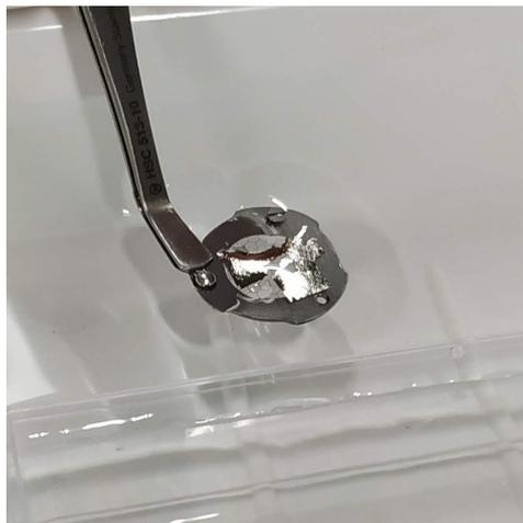
*Figure 60: A photograph of a 50 nm thick tungsten dummy foil that is being caught from the water by a molybdenum grid ring.*
