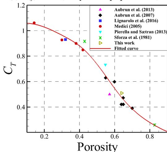
**Figure 6.** Thrust coefficient of porous plates as a function of porosity in literature.
