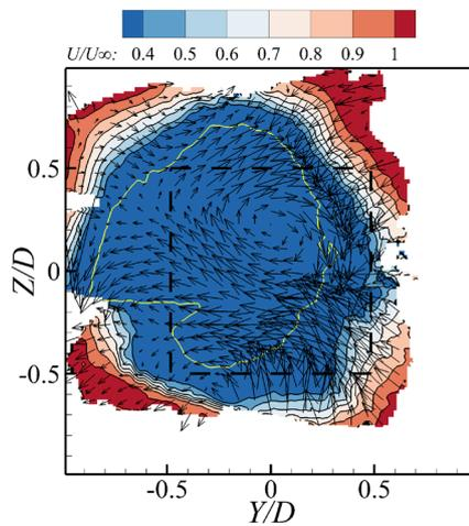
**Figure 10.** Stream-wise velocity contour and in-plane velocity vectors of the plate in yaw, the yellow line denoted the zero velocity. ( $X/D = 1.5$ , yaw angle =  $15^\circ$ )
