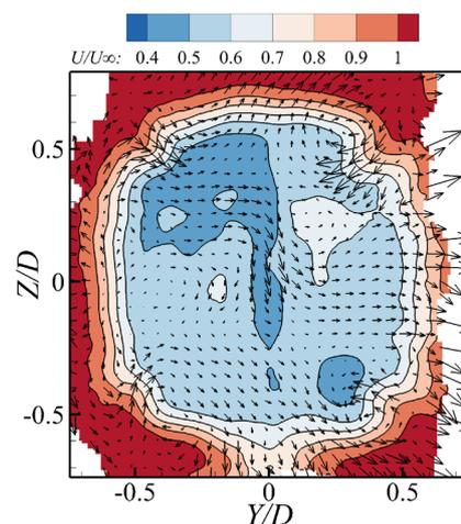
**Figure 9.** Stream-wise velocity contour and in-plane velocity vectors of the plate perpendicular to the flow ( $X/D = 1.5$ )
