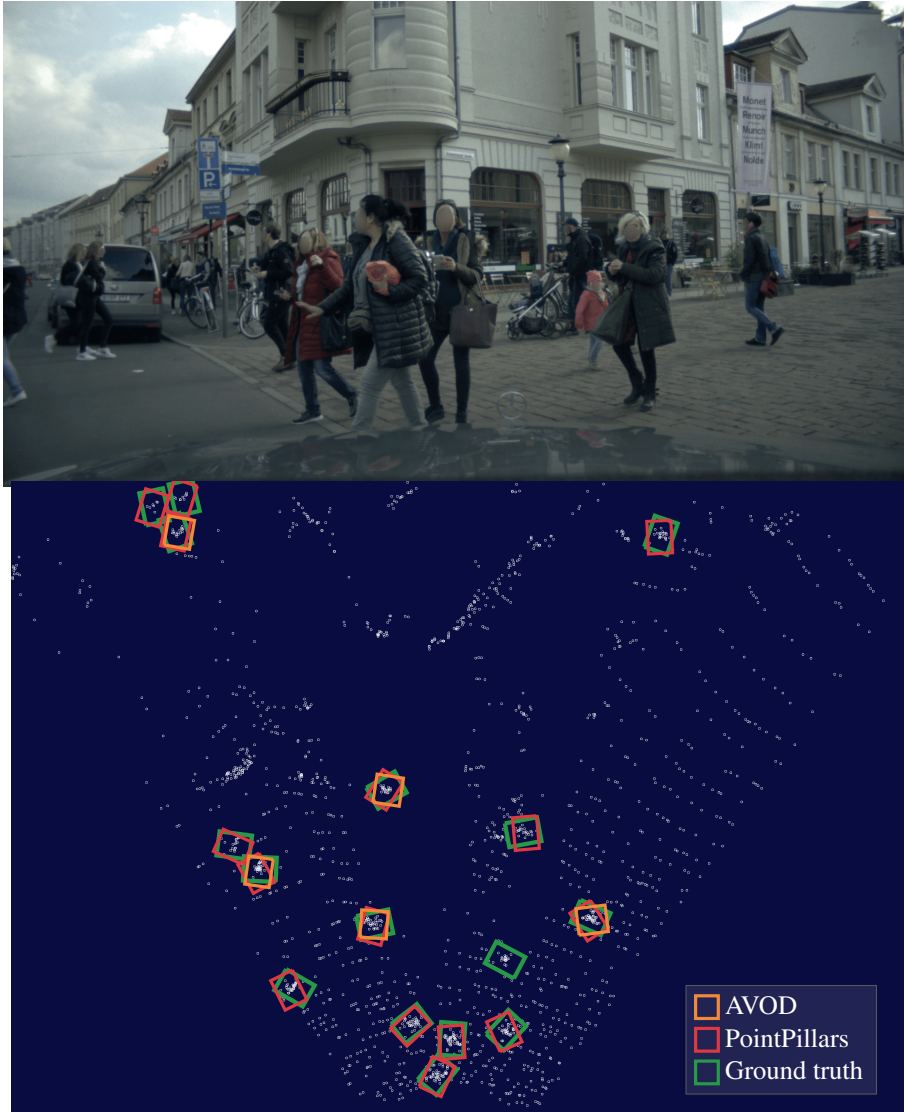
Figure 3.1: An example of the predicted bounding boxes of PointPillars [16] and AVOD [17] on a scene from the EuroCity Persons 2.5D [19], along with the annotated ground truth.
