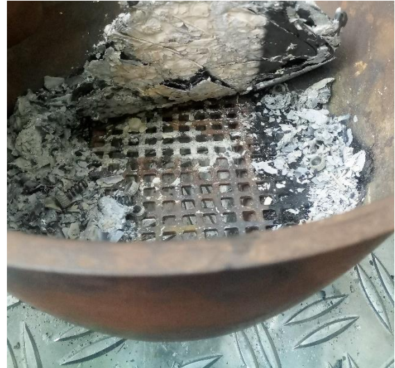
Figure 14. Zamak and coating residue in bowl from melting setup #1 sticking to the sides
