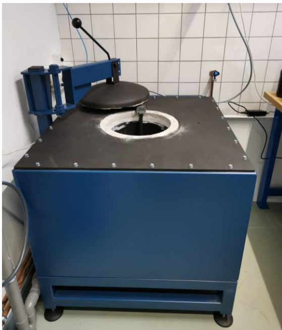
Figure 7. The induction furnace used to melt the Zamak
