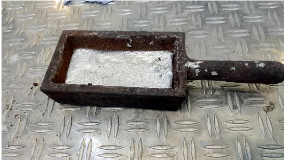
Figure 5. Ingot mold containing a Zamak ingot.
