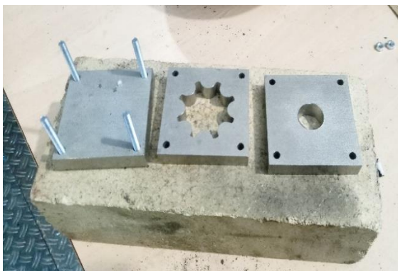
Figure 22. First iteration of the rotation knob mold disassembled
