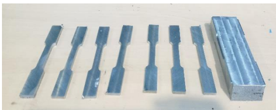
Figure 23. Dogbone samples made from Ingot S1-A
