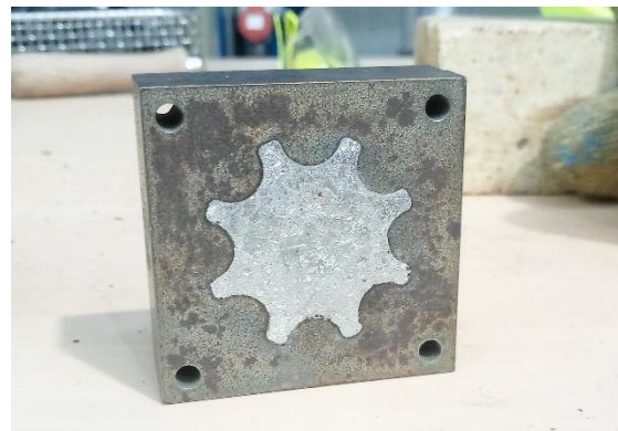
Figure 31. Rotation knob stuck in mold shape slab
