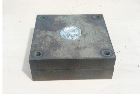
Figure 30. Top and middle mold slabs sticking together, rotation knob stuck in mold
