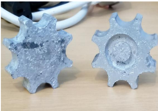
Figure 29. Zamak castings of the rotation knob. Pictured left: first iteration; Pictured right: second iteration.
