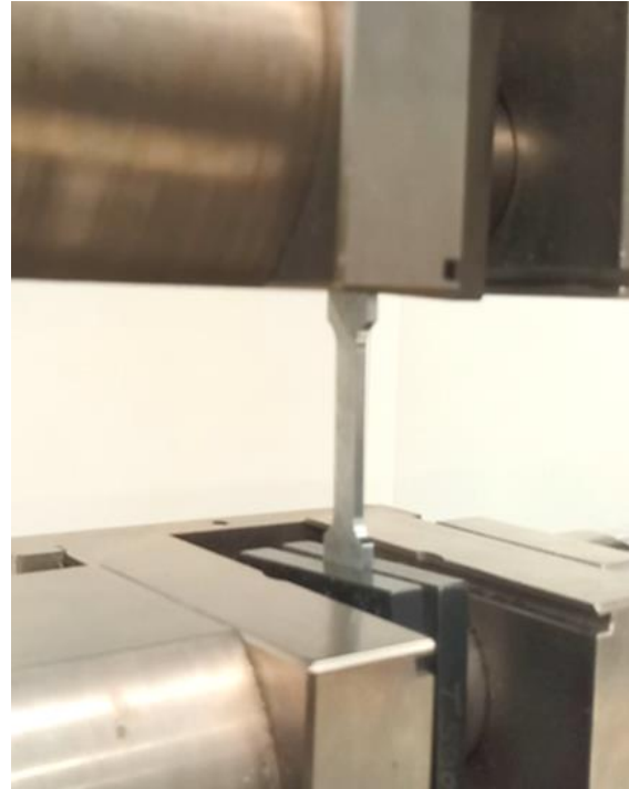
Figure 25. Tensile test with a dogbone sample
