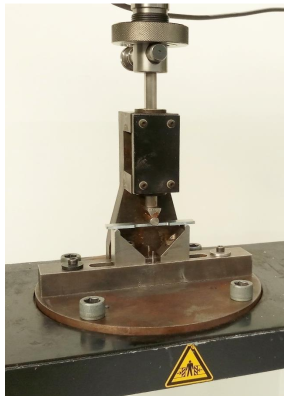
Figure 26. 3-point bend test with a dogbone sample
