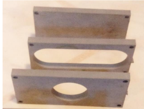
Figure 19. Second iteration ingot mold
