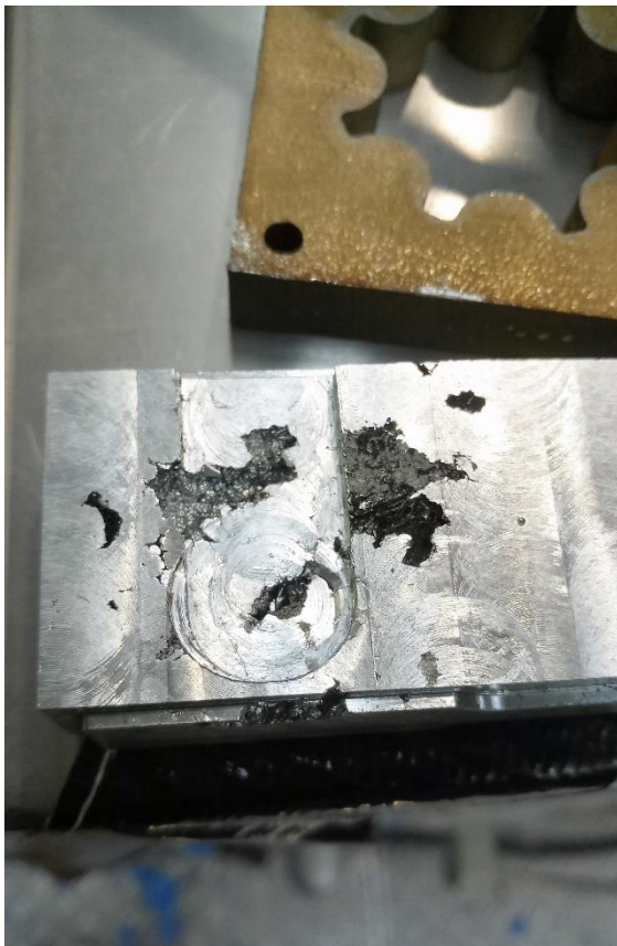
Figure 32. Porosity defects found after machining of Ingot S1-A
