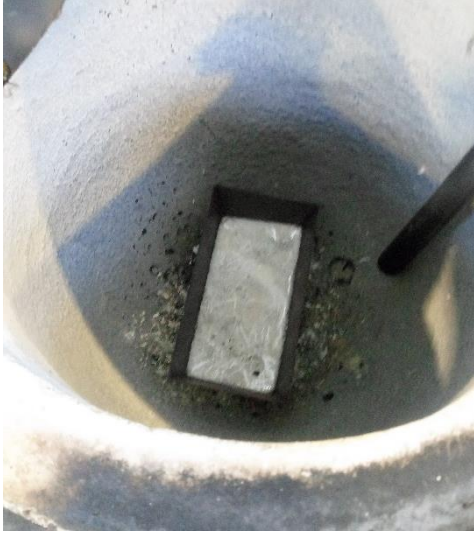
Figure 9. Visual observation of amount of Zamak in mold
