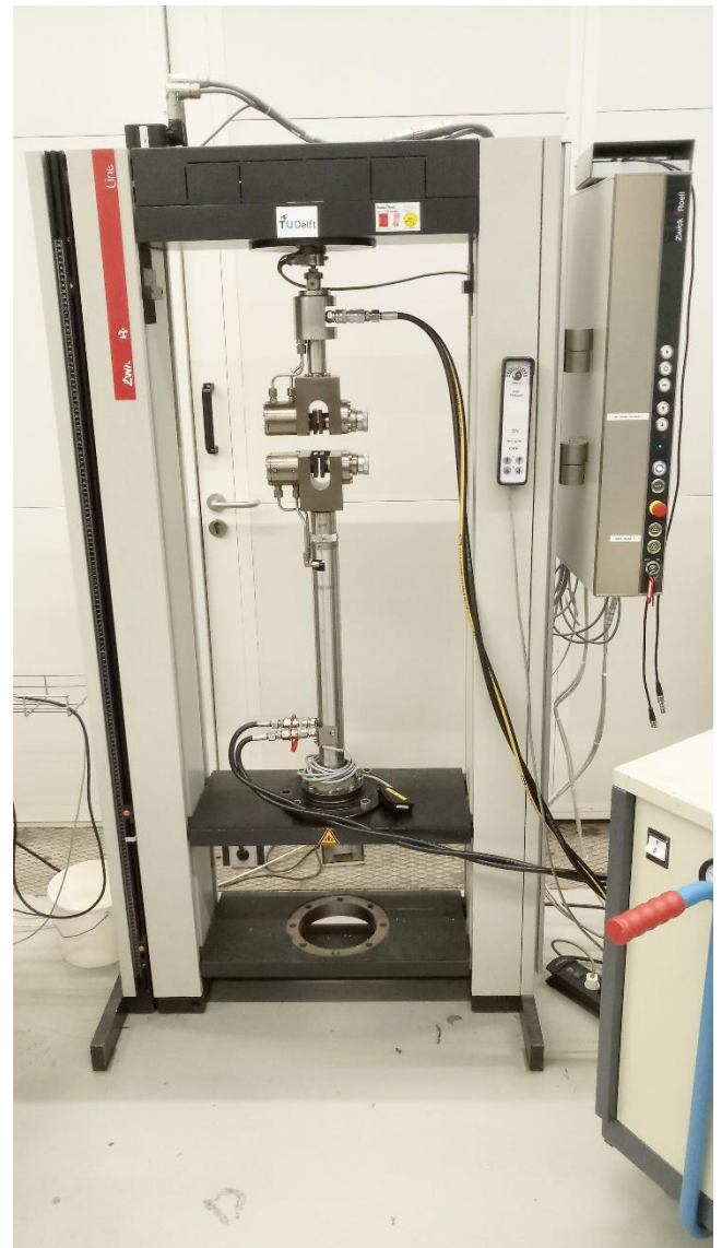
Figure 24. The Zwick/Roell AllroundLine machine used for mechanical testing
