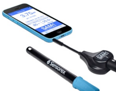
Figure 1.1 – Example of mobile sensing devices. A plug-in sensor is used to measure pH, Oxidation Reduction Potential, temperature and Electric Conductivity.
