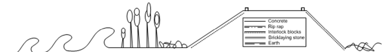
Figure 2-13 Schematic cross section of sea dike #2
