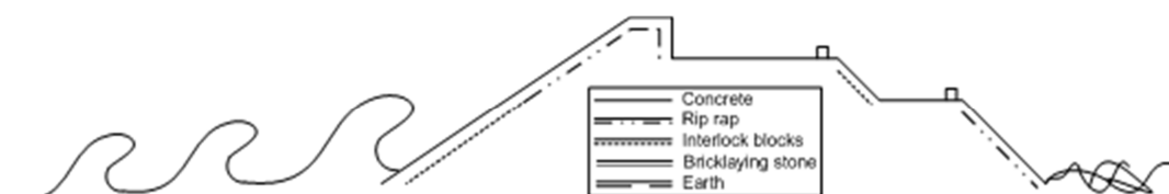
Figure 2-4 Schematic cross section of test dike #1 on Cat Hai Island
