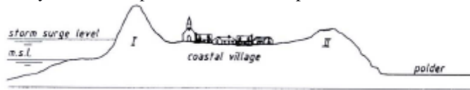
Figure 4: Situation in which erosion should be controlled
