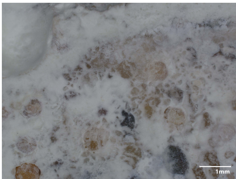
Figure A.4: A magnified image of the efflorescent crust on the surface of an Mortar-F specimen (corresponding to Figure 6.6, left column). The image was acquired at the end of the third absorption-drying cycle.
