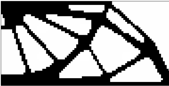
(b) Solution from homogeneous input after 1000 steps. C \approx 94.86
