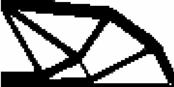
(c) Design after 1000 steps of SIMP, filtered C \approx 90.50
