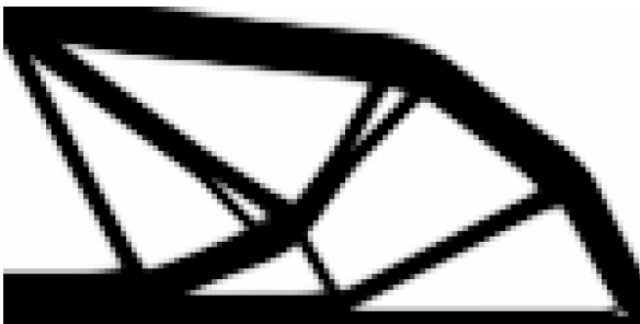
(a) Design after 1000 steps of SIMP C \approx 94.54
