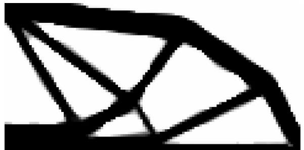
(b) Best design after post-processing C \approx 93.67
