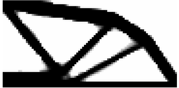
(b) Best design after post-processing C \approx 94.33
