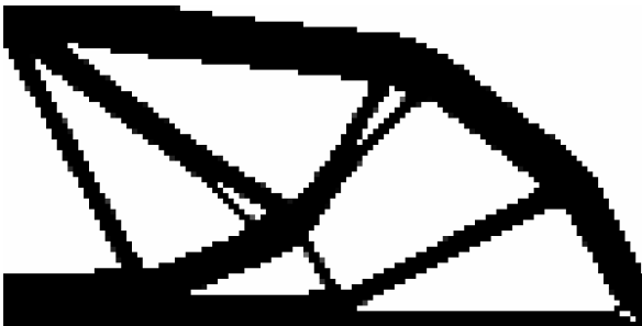
(c) Design after 1000 steps of SIMP, filtered C \approx 90.77
