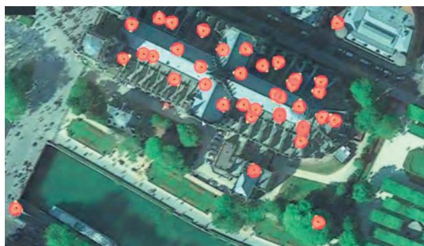
▲ Figure 5: In this aerial view of Notre-Dame Cathedral in Paris, orange circles represent the scan positions during the 2010 TLS survey.
