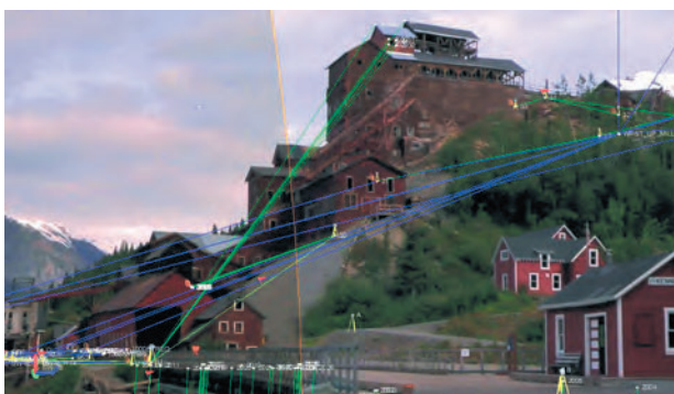
▲ Figure 4: A georeferenced photo mosaic of the Kennecott mill viewed from the valley floor, created using Trimble VISION.
