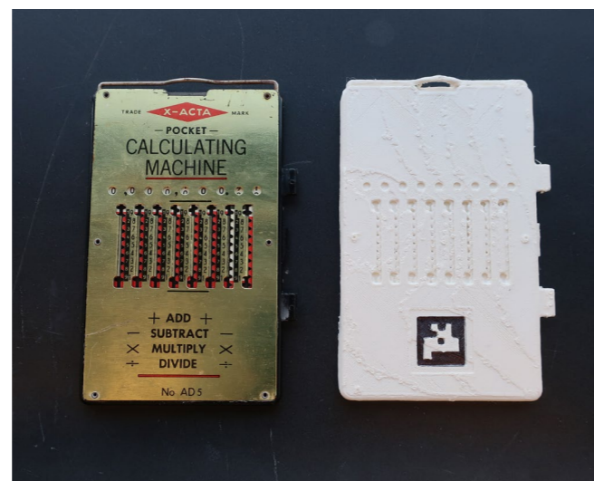
Figure 42. The original artifact (left) and its 3D printed replica with integrated visual marker (right).
