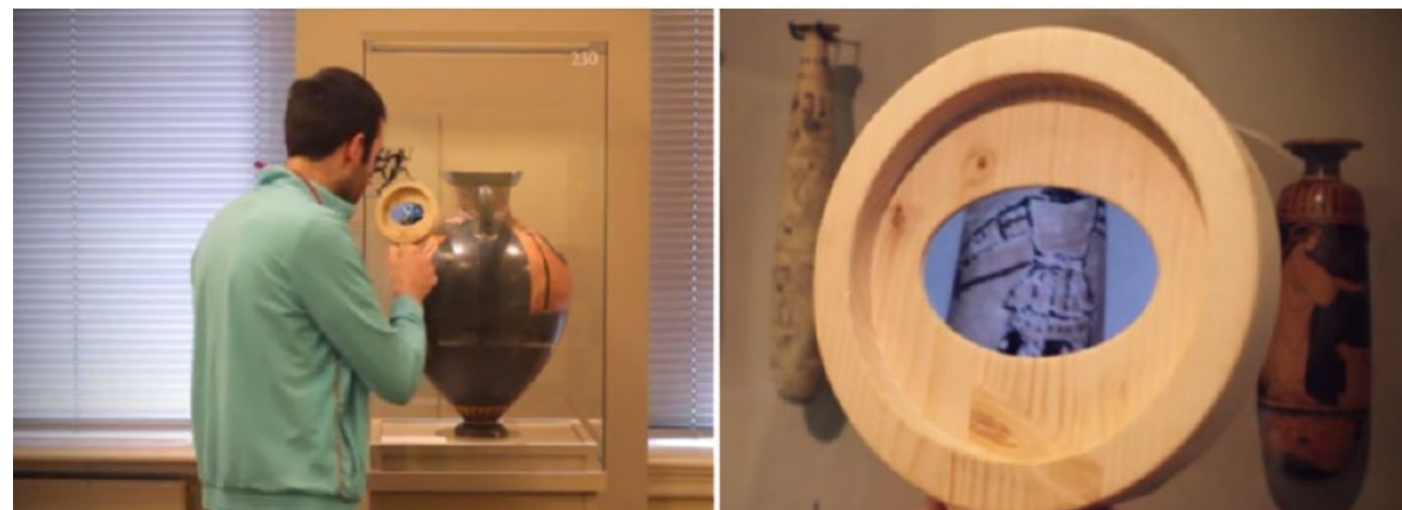
Figure 9. The Loupe is an AR wooden magnifying lens embedded with an iPhone. It enables visitors to examine objects up close and access extra digital content (Van Der Vaart & Damala, 2015; Zancanaro et al., 2015).
