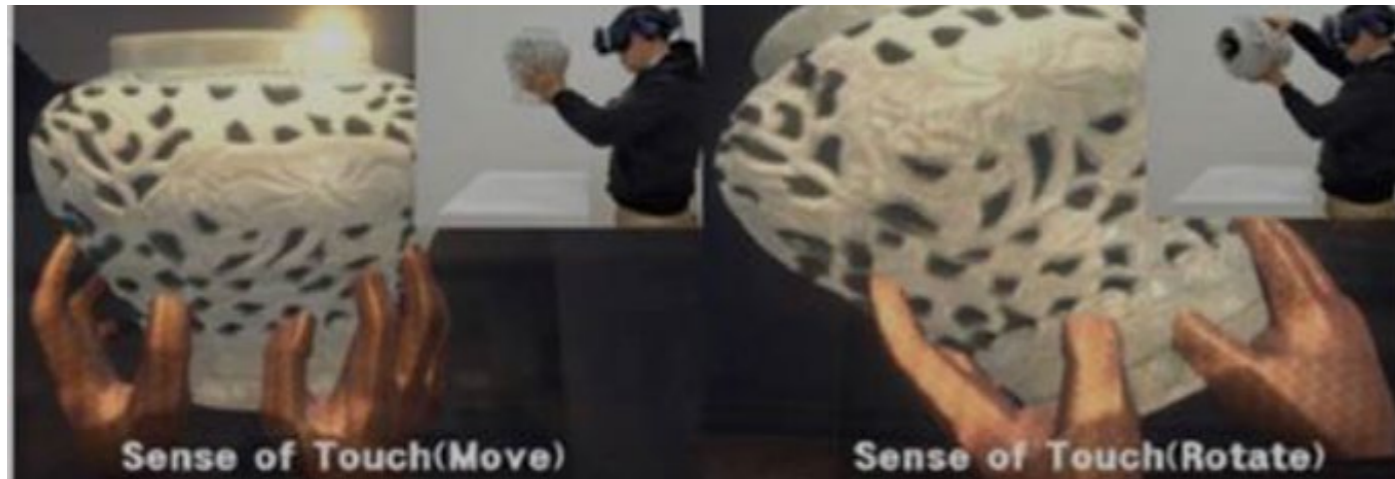
Figure 18. This system allows users to naturally manipulate virtual objects using 3D-printed replicas (Kim et al., 2023).
