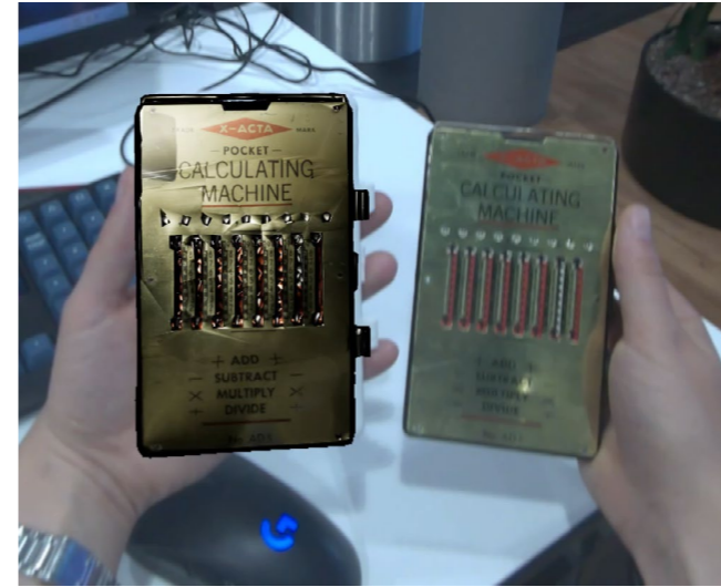
Figure 43. A 3D scan attached to a physical replica with an integrated visual marker (left) and the original artifact (right).
