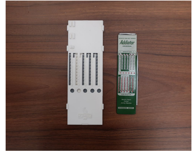
Figure 44. A 3D printed adder (left) and the original artifact (right).
