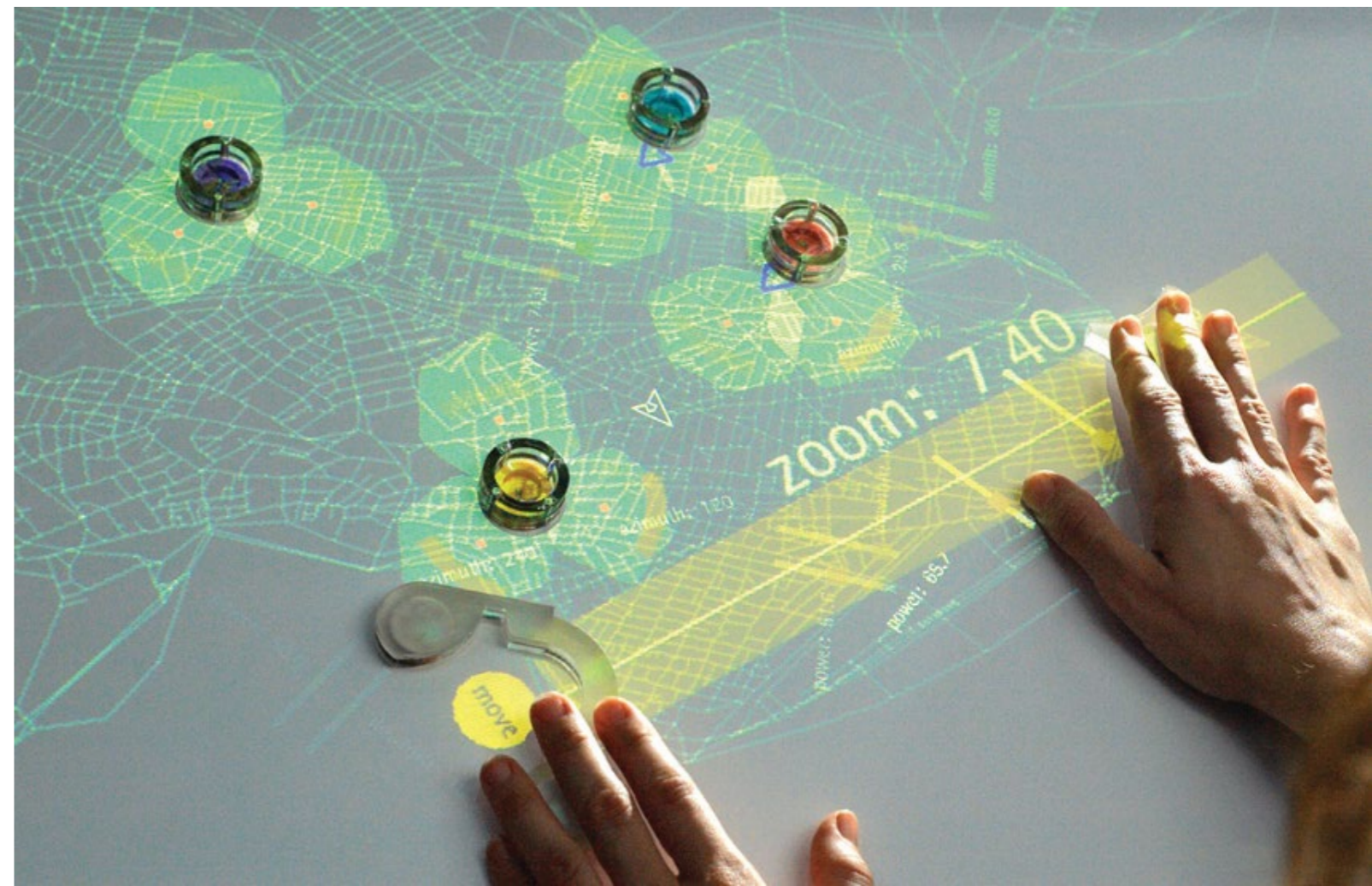
Figure 14. PICO is a tabletop interaction surface that uses electromagnets to track and move small objects, allowing users to physically interact with computational optimization processes, such as cellphone tower placement (Ishii et al., 2012).
