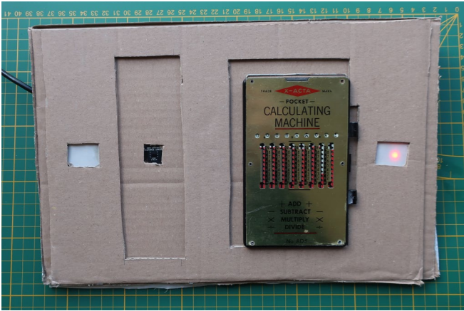
Figure 48. ToF/light sensor prototype: The calculators are recognized and lights will turn on if they're placed in the correct slots.
