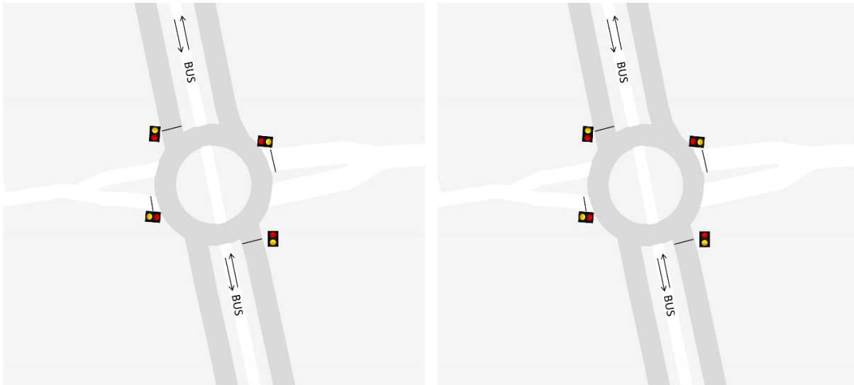
Figure 12 Two solutions for throughabouts with traffic signals for entering traffic (left) and traffic signals for conflicting traffic (right)
