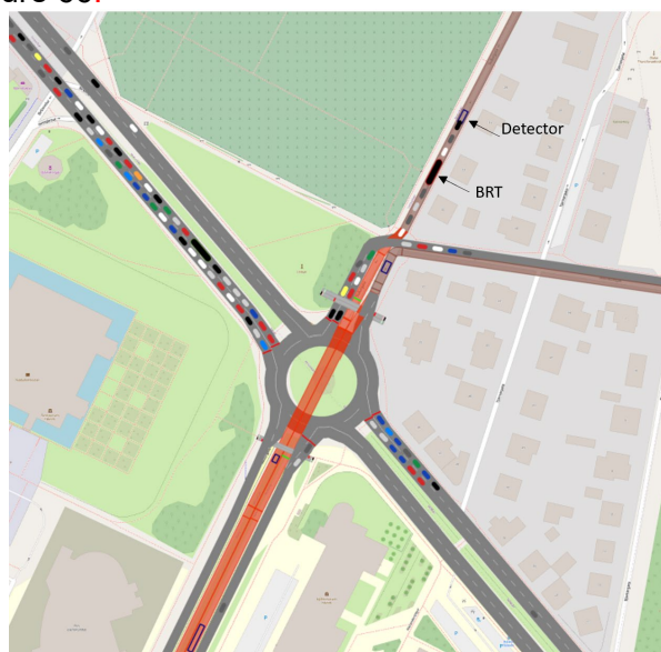
Figure 66 Gridlock starting after a bus passed the detector but is stuck in a queue
