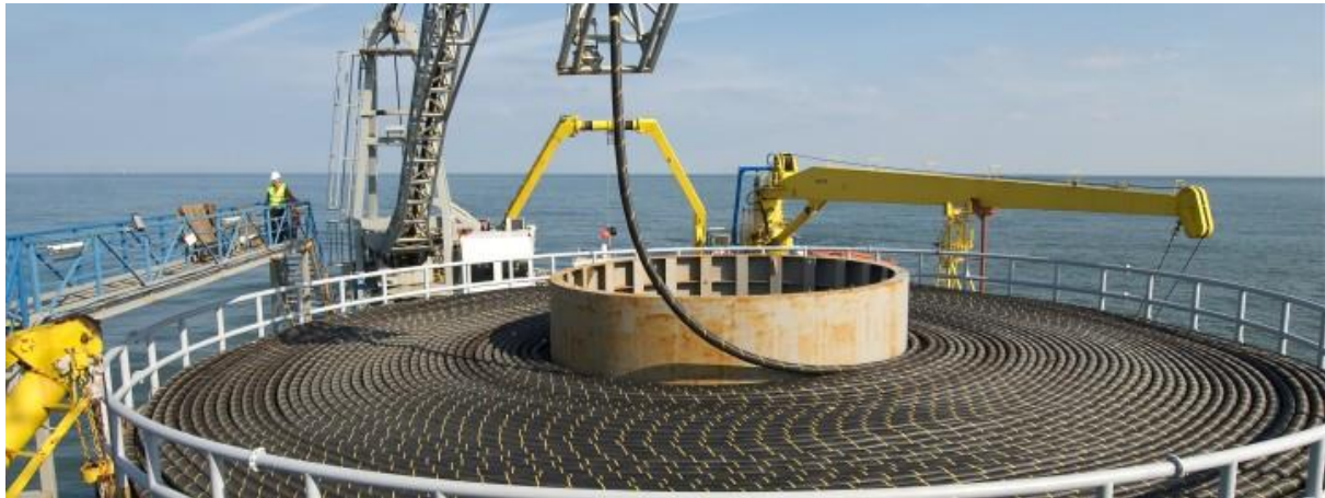
Figure 1-3: Storage of offshore power cable in carousel [5]
