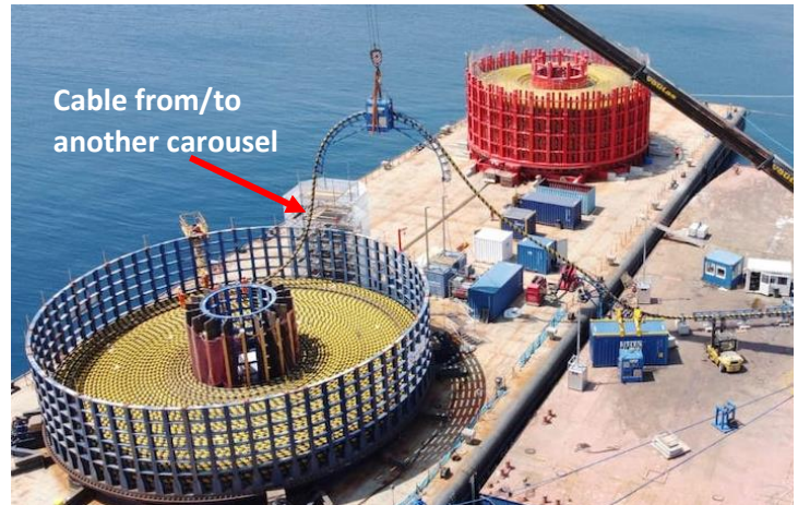
Fig. 1: General cable transfer / carousel (un)spooling setup [8]
