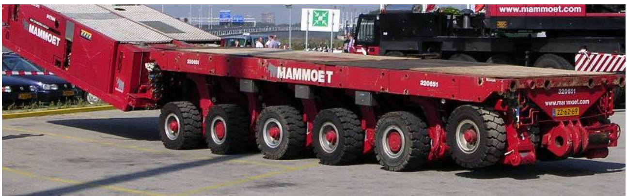
Figure 2-13: Mammoet SPMT with 6 axle lines [28]
