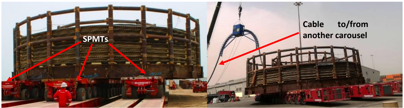
Figure 1-8: 1300t capacity carousel transfer to barge [11]
