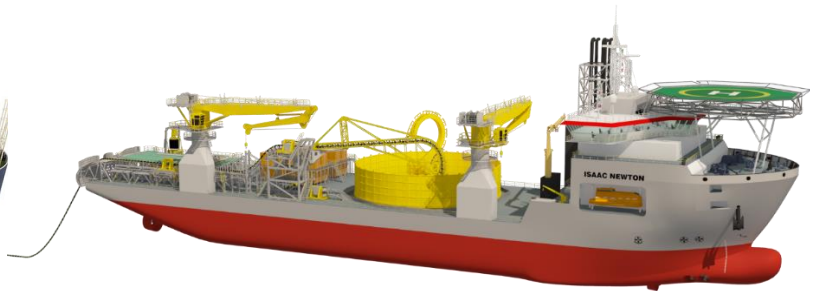
Figure 2-7: Cable installation vessel [17]
