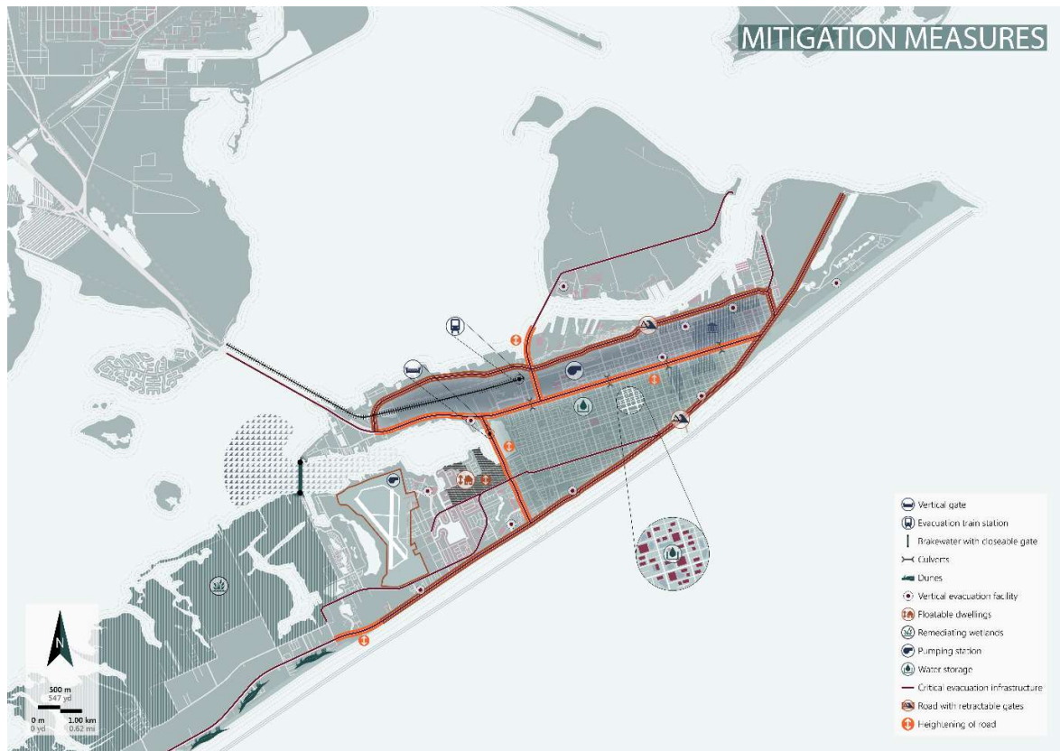
Figure 45 Integral design of mitigation measures
