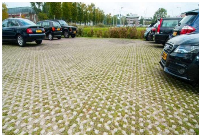
Figure 83 Parking lot with permeable concrete (Michon, 2018)
