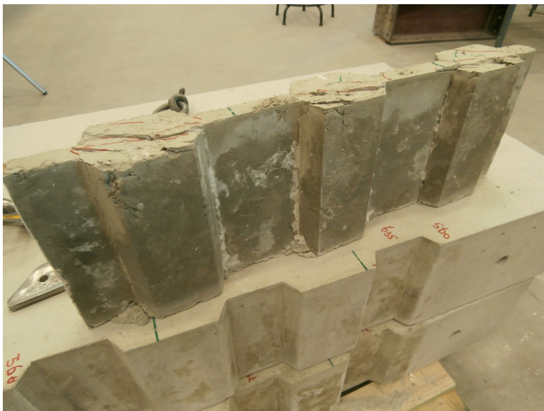
Figure E.2: Specimen 1-4: Dismantled specimen (Steel Fibre Reinforced Mortar)
