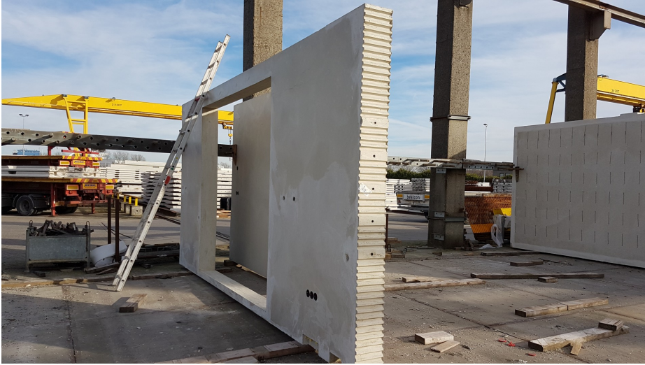
Figure 3.6: Precast concrete element with a profiled edge side for the Aligned small shear key
