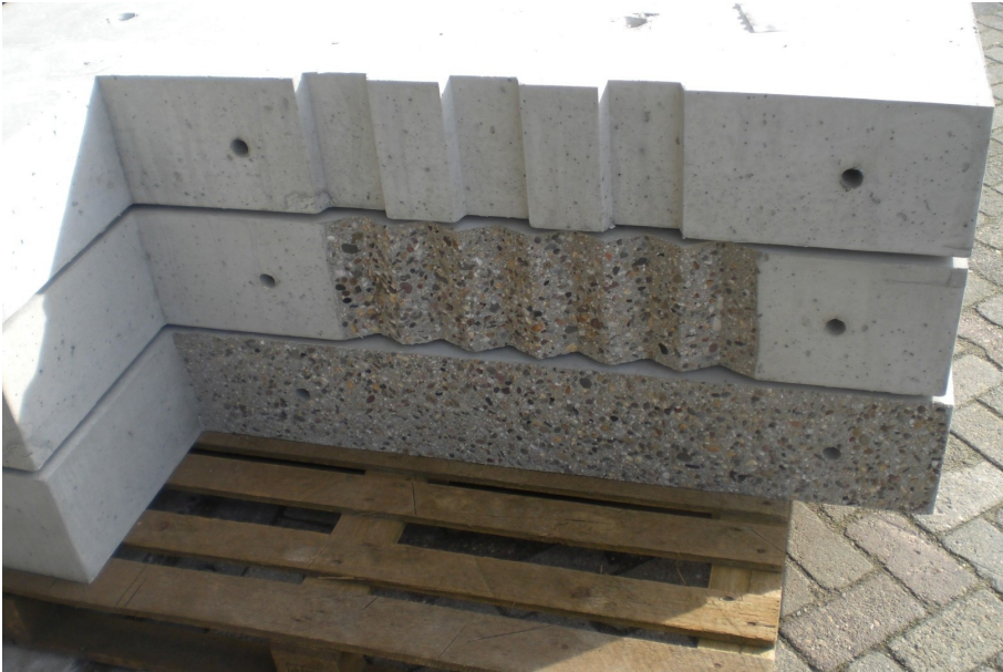
Figure 3.8: Shear keys for Staggered shear key connection (upper element), Serrated waterjetted shear connection (middle element) and Plain waterjetted shear connection (bottom element)
