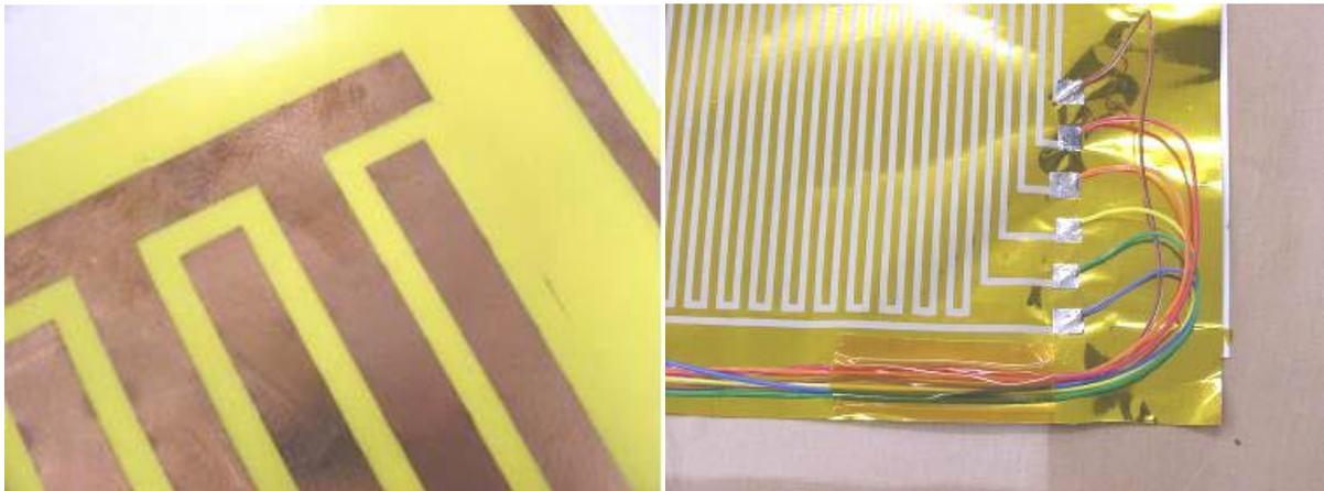
Figure 23: (Left) Etched copper on Polyurethane Coated Nylon. (Right) Printed Conductive Ink on Aluminized Kapton™. [Source: 69]
