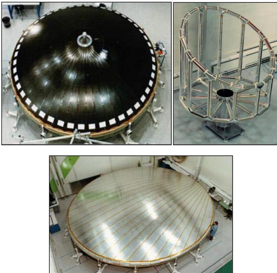
Figure 5: (Top left) VLBI antenna. (Top right) Inflatable sun shade structure. (Bottom) Inflatable communications reflector antenna [Source: 6]
