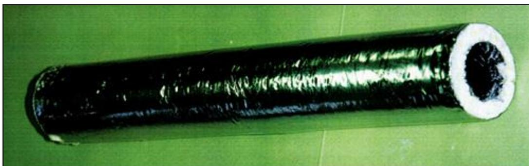
Figure 19: Inflating cured-pipe by the foaming method [Source: 53]
